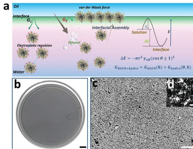
**Fig. 3** (a) Schematic illustration of spiky Au@Ag NP monolayer films acquired at the oil–water interface. Optical photograph (b), SEM (c) and TEM (d) images of spiky Au@Ag NPs monolayer film. The scale bar is 1 cm (b), 20 μm (c) and 100 nm (d), respectively.
