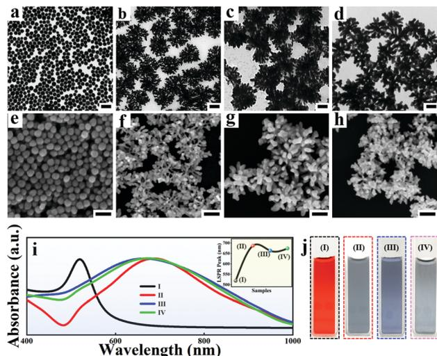
**Fig. 2** TEM and SEM images of Au NPs (a and e), spiky AuNPs (b and f), spiky Au@Ag NPs (c and g) and etched-spiky Au@Ag NPs (d and g). (i and j) UV-vis spectra and optical photographs of the aqueous solution of Au NPs (I), spiky AuNPs (II), spiky Au@Ag NPs (III) and etched-spiky Au@Ag NPs (IV) (inset: LSPR peak location of the proposed four different NPs). The scale bar is 50 nm.
