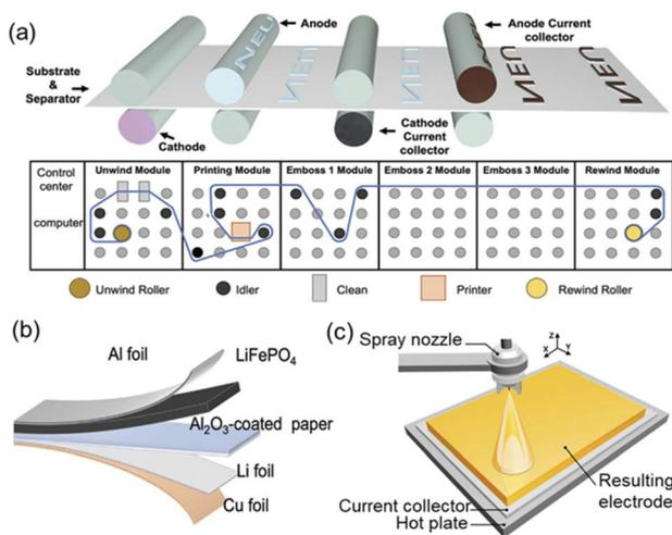
Fig. 6 (a) Schematic diagram of flexographic printing and (b) a thin-film lithium metal battery based on the flexographic printed  $\text{LiFePO}_4$  cathode. Reproduced with permission from ref. 62, Copyright© 2022, Wiley-Blackwell. (c) Schematic diagram of spray printing for preparing thin film electrodes of LIBs. Reproduced with permission from ref. 63, Copyright© 2018, Elsevier Ltd.
