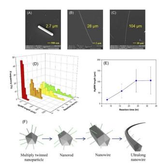
SEM images illustrating the effect of reaction time 4 h (A), 8 h and (B), 24 h (C) and length distribution of the AgNWs (D) and average size of the AgNWs (E) with respect to reaction time and (F) schematic illustration of ultralong nanowire formation.
