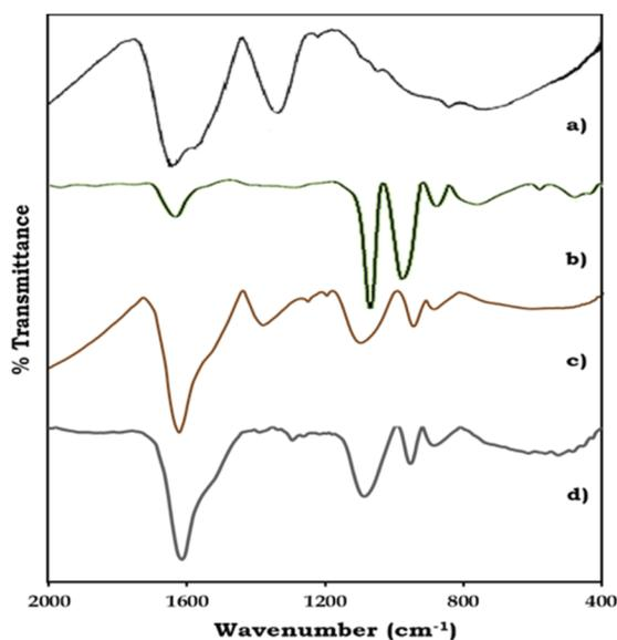
Fig. 2 FT-IR spectra of (a) ZrO<sub>2</sub>, (b) PMA, (c) PMA/ZrO<sub>2</sub> and (d) Pd-PMA/ZrO<sub>2</sub>.
