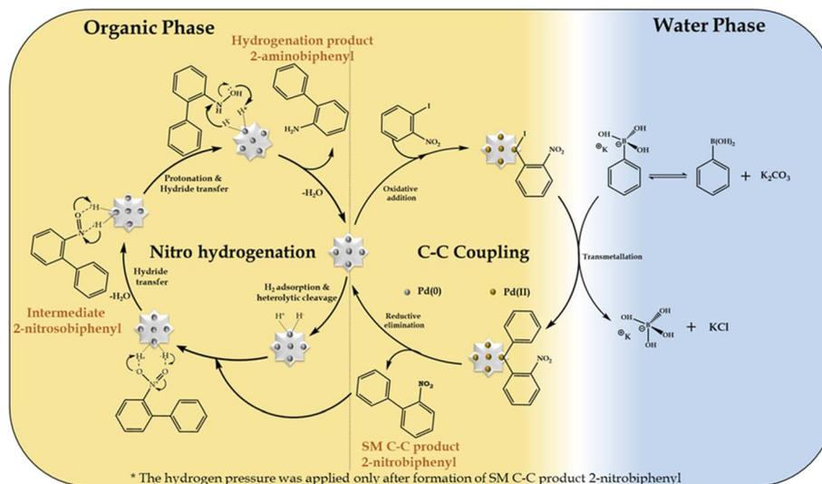
Scheme 4 Plausible mechanism for the Suzuki–Miyaura cross-coupling/nitro hydrogenation reaction.
