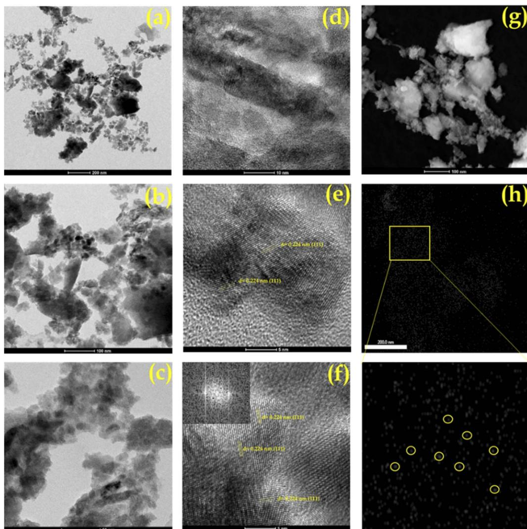
Fig. 7 (a–c) TEM images, (d–f) HRTEM images and (g) HAADF STEM of Pd-PMA/ZrO<sub>2</sub> and (h) elemental mapping of Pd.
