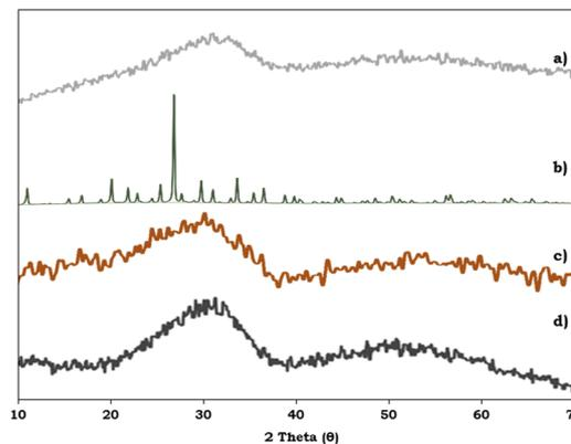
Fig. 6 Powder XRD of (a) ZrO<sub>2</sub>, (b) PMA, (c) PMA/ZrO<sub>2</sub> and (d) Pd-PMA/ZrO<sub>2</sub>.
