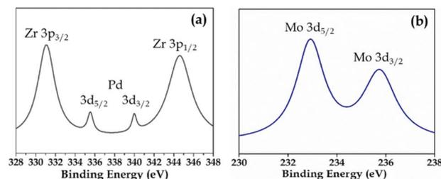
Fig. 12 XPS of (a) Pd and (b) Mo in R-PMA/ZrO<sub>2</sub>.
