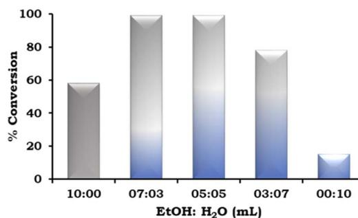
Fig. 9 Effect of EtOH : H<sub>2</sub>O. Reaction condition: 1-iodo-2-nitrobenzene (1.96 mmol), phenylboronic acid (2.94 mmol), catalyst amount (20 mg), K<sub>2</sub>CO<sub>3</sub> (3.92 mmol), time (2 h) and temp. (90 °C).
