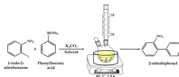
Scheme 2 Schematic illustration of the Suzuki–Miyaura cross-coupling reaction.
