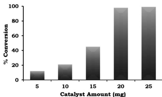
Fig. 8 Effect of catalyst amount. Reaction conditions: 1-iodo-2-nitrobenzene (1.96 mmol), phenylboronic acid (2.94 mmol), K<sub>2</sub>CO<sub>3</sub> (3.92 mmol), EtOH : H<sub>2</sub>O (5 : 5 mL), time (2 h), and temp. (90 °C).
