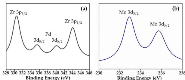
Fig. 4 XPS of (a) Pd and (b) Mo in PMA/ZrO<sub>2</sub>.
