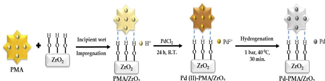
Scheme 1 Synthesis of zirconia-supported phosphomolybdic acid-stabilized Pd SAC.
