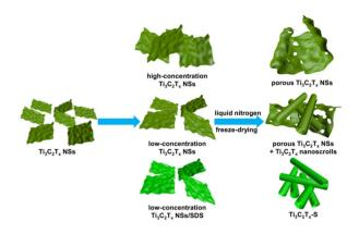
Fig. 4 Schematic illustration for synthesizing different Ti<sub>3</sub>C<sub>2</sub>T<sub>x</sub> structures through regulation of concentrations and electronegativity.
