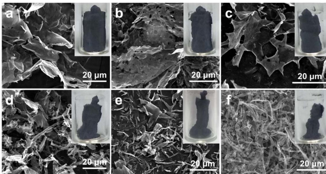
Fig. 2 FESEM images and digital pictures (the insets) of (a)  $\text{Ti}_3\text{C}_2\text{T}_x-2.0$ , (b)  $\text{Ti}_3\text{C}_2\text{T}_x-1.0$ , (c)  $\text{Ti}_3\text{C}_2\text{T}_x-0.8$ , (d)  $\text{Ti}_3\text{C}_2\text{T}_x-0.5$ , (e)  $\text{Ti}_3\text{C}_2\text{T}_x-0.2$  and (f)  $\text{Ti}_3\text{C}_2\text{T}_x-0.1$  samples.
