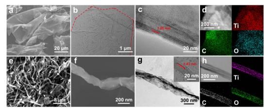
Fig. 1 (a) FESEM, (b) TEM, (c) HRTEM, and (d) STEM and corresponding EDX mapping images of  $Ti_3C_2T_x$  NSs; (e and f) FESEM, (g) TEM and HRTEM (the inset in panel (g)), and (h) STEM and corresponding EDX mapping images of  $Ti_3C_2T_x$ -S.
