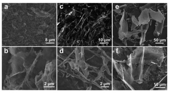
Fig. 3 FESEM images of (a and b)  $Ti_3C_2T_x$ -C and (c and d)  $Ti_3C_2T_x$ -P frozen with liquid  $N_2$ , and (e and f)  $Ti_3C_2T_x$ -r.
