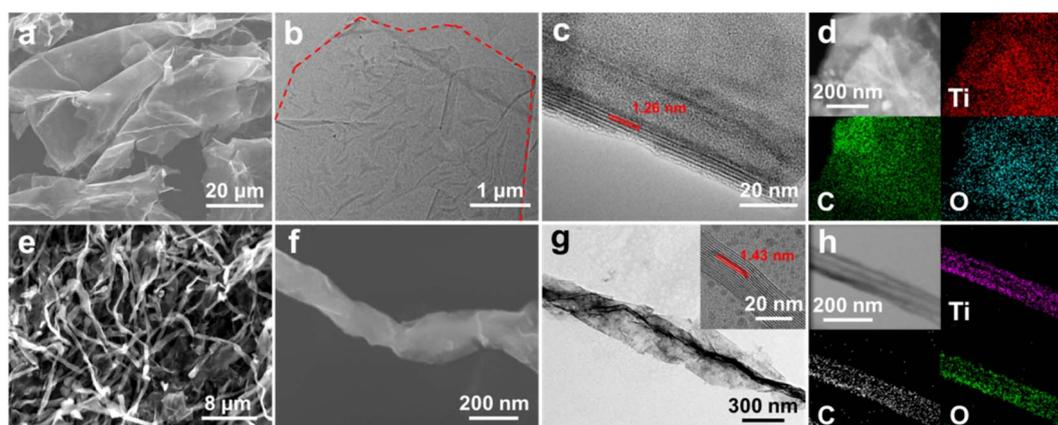
Fig. 1 (a) FESEM, (b) TEM, (c) HRTEM, and (d) STEM and corresponding EDX mapping images of  $\text{Ti}_3\text{C}_2\text{T}_x$  NSs; (e) and (f) FESEM, (g) TEM and HRTEM (the inset in panel (g)), and (h) STEM and corresponding EDX mapping images of  $\text{Ti}_3\text{C}_2\text{T}_x\text{-S}$ .
