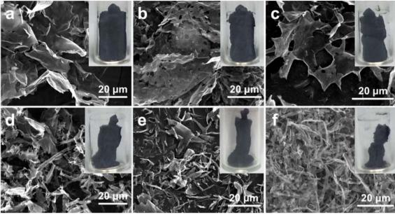
Fig. 2 FESEM images and digital pictures (the insets) of (a)  $Ti_3C_2T_x-2.0$ , (b)  $Ti_3C_2T_x-1.0$ , (c)  $Ti_3C_2T_x-0.8$ , (d)  $Ti_3C_2T_x-0.5$ , (e)  $Ti_3C_2T_x-0.2$  and (f)  $Ti_3C_2T_x$ -0.1 samples.
