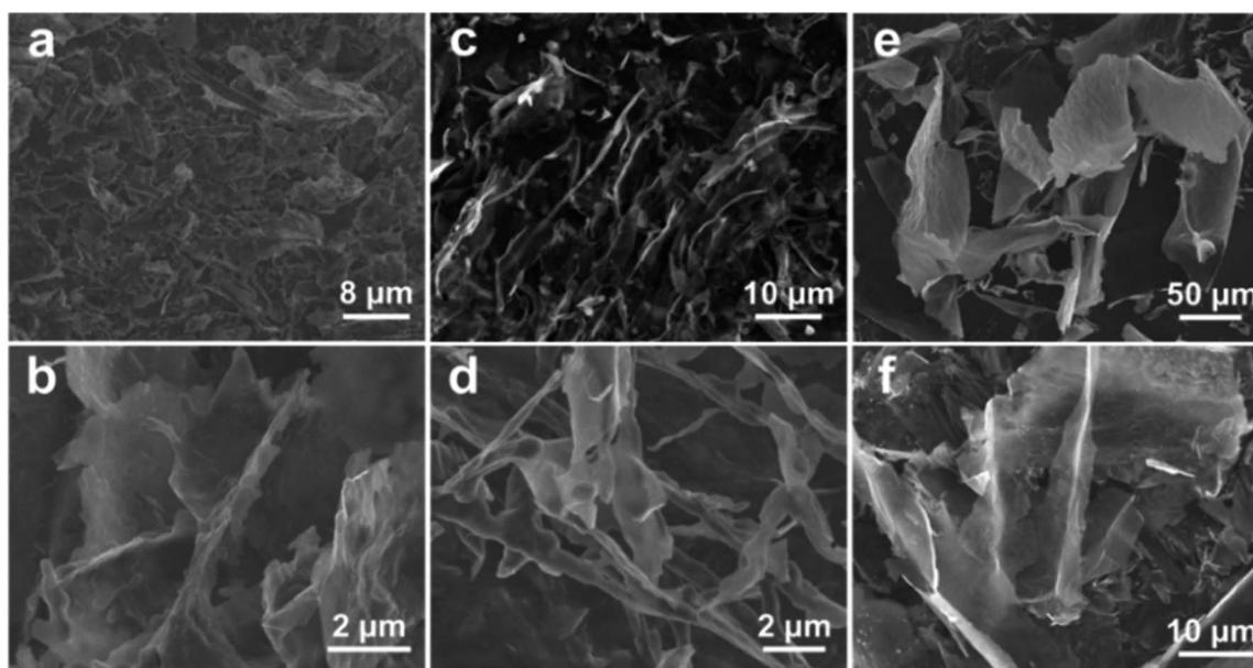
Fig. 3 FESEM images of (a and b)  $\text{Ti}_3\text{C}_2\text{T}_x\text{-C}$  and (c and d)  $\text{Ti}_3\text{C}_2\text{T}_x\text{-P}$  frozen with liquid  $\text{N}_2$ , and (e and f)  $\text{Ti}_3\text{C}_2\text{T}_x\text{-r}$ .
