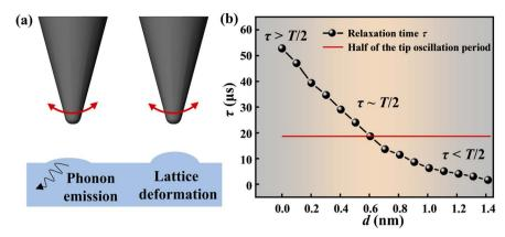
Fig. 3 (a) Model schematic diagram. The oscillation of the tip can cause the atoms on the surface of the sample to vibrate, which can excite phonons and even cause lattice deformation; (b) the mean relaxation time of atomic vibration on the graphite surface varies with the tip-sample distance. At  $d \sim 0.6$  nm, the mean relaxation time is equivalent to half of the tip oscillation period, which induces significant hysteretic behavior and dissipation peaks.
