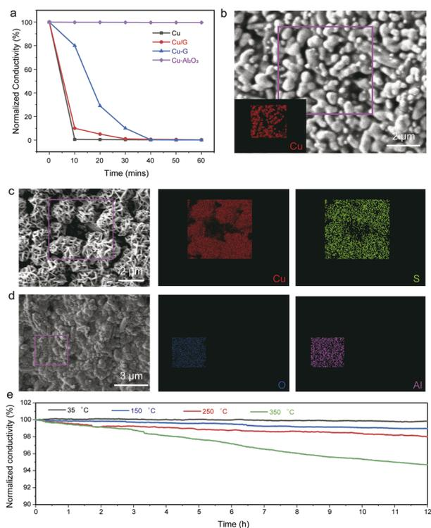
Fig. 4 Cu-based conductor performances under sulfurous atmosphere. (a) Conductivity changes of the Cu-based conductors (Cu, Cu/G, Cu-G and Cu-Al<sub>2</sub>O<sub>3</sub>) at 150 °C under sulfurous atmosphere. (b) SEM image of Cu before the test. Inset is the EDS mapping. (c) SEM and EDS images of Cu after the test. (d) SEM and EDS images of Cu-Al<sub>2</sub>O<sub>3</sub> after the test. (e) Conductivity changes of Cu-Al<sub>2</sub>O<sub>3</sub> at different temperatures for 12 h.
