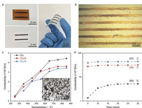
Fig. 3 Conductivity of the printed Cu-based conductor. (a) Picture of the printed Cu conductor on flexible Kapton®, paper and ceramic substrate *via* direct writing. (b) Ink-jet printing of the Cu conductor on the Kapton® substrate. (c) Electrical conductivity as a function of sintering temperature. Inset is an SEM image of the Cu NPs after sintering at 850 °C. (d) The plot of Cu NP conductivity *versus* sintering time at 250 °C, 550 °C and 850 °C.
