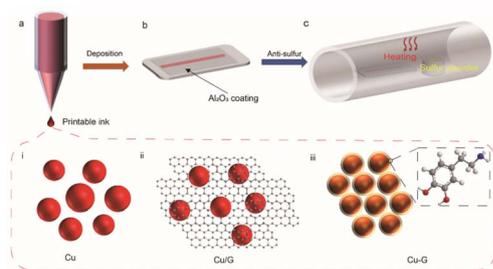
Fig. 1 Schematic of the Cu-based conductor for sulfur corrosion resistance. (a) Printing of the Cu-based conductors: Cu NPs (i), Cu/G (ii), and Cu-G (iii). (b) Cu-based conductor with a thin  $\text{Al}_2\text{O}_3$  layer coating. (c) Schematic of *in situ* measurement under a sulfurous atmosphere at different temperatures.
