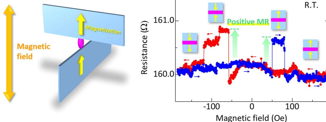
Fig. 7 MR effect in Ni<sub>78</sub>Fe<sub>22</sub>/C8-BTBT (4 nm)/Ni<sub>78</sub>Fe<sub>22</sub> nanojunctions with a junction area of 42 × 42 nm<sup>2</sup> at room temperature. The P and AP configurations of magnetization in the two electrodes are also shown. A positive MR effect, that is,  $R_{AP} > R_P$ , is clearly observed.
