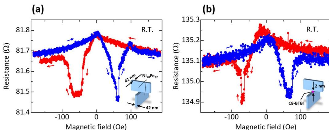
Fig. 6 MR effect in (a)  $\text{Ni}_{78}\text{Fe}_{22}/\text{Ni}_{78}\text{Fe}_{22}$  and (b)  $\text{Ni}_{78}\text{Fe}_{22}/\text{C8-BTBT}$  (2 nm)/ $\text{Ni}_{78}\text{Fe}_{22}$  nanojunctions with a junction area of  $42 \times 42 \text{ nm}^2$  at room temperature. The blue (red) plots represent the results obtained under the forward (reverse) sweeping field.
