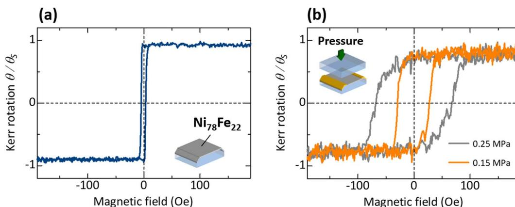
Fig. 5 Magnetization curves of the  $\text{Ni}_{78}\text{Fe}_{22}$  (42 nm) film (a) before and (b) after thermal pressing. The coercivity increases to 29 and 68 Oe by increasing the applied pressure to 0.15 and 0.25 MPa, respectively, during the thermal pressing process.
