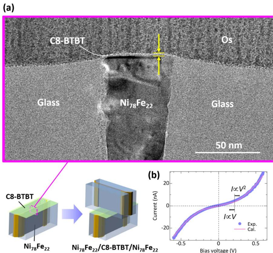
Fig. 4 (a) Cross-sectional TEM image obtained for 2 nm thick C8-BTBT films on the polished surface of the glass/ $\text{Ni}_{78}\text{Fe}_{22}$  (42 nm)/glass substrates. (b)  $I$ - $V$  characteristics of the polished  $\text{Ni}_{78}\text{Fe}_{22}$  edge after the formation of C8-BTBT films. The nonlinear behavior can be explained in terms of the SCLC.
