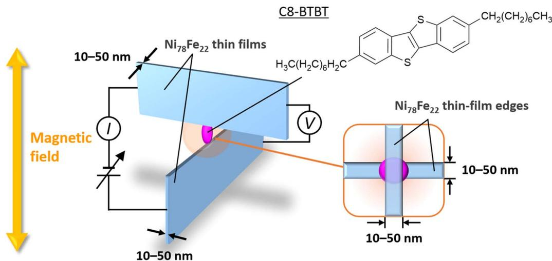
Fig. 1 Schematic of  $\text{Ni}_{78}\text{Fe}_{22}/\text{C8-BTBT}/\text{Ni}_{78}\text{Fe}_{22}$  nanojunctions utilizing thin-film edges. The nanojunction consists of C8-BTBT molecules sandwiched between two  $\text{Ni}_{78}\text{Fe}_{22}$  thin films with crossed edges. The junction area is determined by the film thickness, that is, 10–50 nm thick films could produce  $10 \times 10$  to  $50 \times 50 \text{ nm}^2$  nanojunctions.
