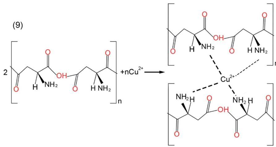
Fig. 6 The chemical reaction equations during CMP.
