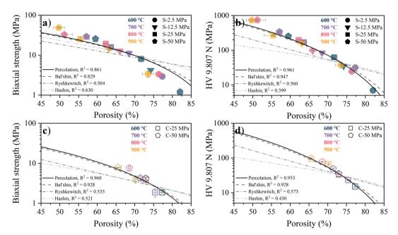
Fig. 9 Biaxial strength (a) and (c) and Vickers hardness HV 9.807 N (b) and (d) over porosity for varying sintering temperatures and pressures for S-and C-sintered COK-12 monoliths as well as corresponding Percolation, Bal'shin, Ryshkewitch, and Hashin fits.
