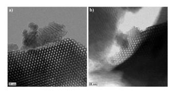
Fig. 2 TEM images of a ground S-sintered COK-12 monolith processed at 50 MPa and 900 °C show the significant preservation of the hexagonally ordered mesopores (a and b) and areas of pore deformation (b).
