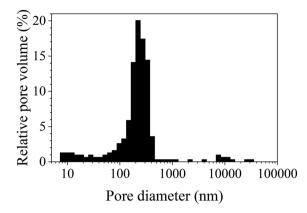
Fig. 8 Pore size distribution histogram obtained from mercury intrusion porosimetry data of S-sintered COK-12 monoliths processed at 12.5 MPa and 800  $^{\circ}$ C.
