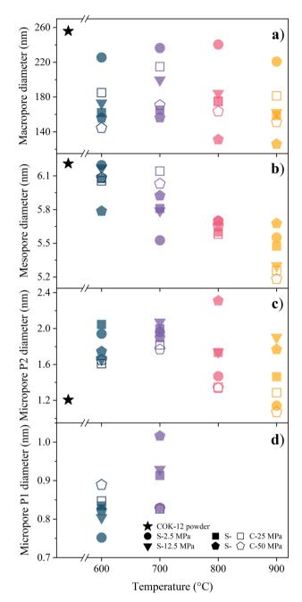
Fig. 5 (a) Macro-, (b) meso-, and (c, d) micropore (P2, P1) diameters obtained from fitting the SAXS data of COK-12 powder and S- and C-sintered monoliths. No P1 micropores were determined for the COK-12 powder and the monoliths sintered at 800 and 900  $^{\circ}$ C.
