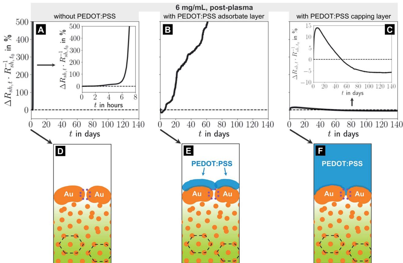
Fig. 4 (A–C): Relative change in sheet resistance  $(R_{sh,t} - R_{sh,t_0})R_{sh,t_0}^{-1} = \Delta R_{sh,t}R_{sh,t_0}^{-1}$  after time  $t$  for electrodes imprinted at  $6 \text{ mg mL}^{-1}$  with different coating finishes. (D–F): illustrations of the apparent microstructures.
