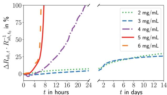
Fig. 1 Relative change in sheet resistance  $(R_{sh,t} - R_{sh,t_0})R_{sh,t_0}^{-1} = \Delta R_{sh,t} R_{sh,t_0}^{-1}$  after time  $t$  for electrodes imprinted at different ink concentrations  $c_{Au}$ . The results of repeated experiments and additional concentrations are shown in Fig. S1 in the ESI.†
