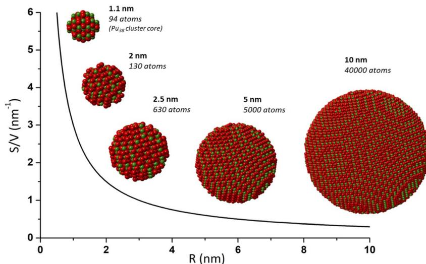
Fig. 1 Scheme illustrating the increasing contribution of surface atoms (surface to volume ratio) toward a shrinking nanoparticle. This effect contributes to providing specific properties to a nanoparticle and is generally observed for a size lower than 10–20 nm. Nanoparticles and calculations of atoms (Pu in green and O in red) were generated with crystal maker software from bulk  $\text{PuO}_2$  and  $\text{Pu}_{38}$  CIF file from Sigmon *et al.*<sup>16</sup>
