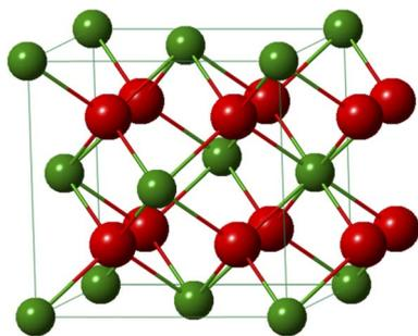
Fig. 11 Cell of the  $\text{PuO}_2$  structure.  $\text{Pu}^{4+}$  and  $\text{O}^{2-}$  are shown in green and red, respectively. In the structure, each O is surrounded by 4 Pu atoms forming tetrahedral sites and each Pu is coordinated by 8 O atoms forming infinite arrays of  $\text{PuO}_8$  cubes.
