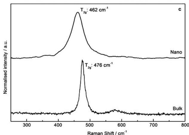
Fig. 9 Raman spectra (488 nm, 1 mW) acquired on PuO<sub>2</sub> nanoparticles (top) and bulk (bottom) in the solid state demonstrating the enlargement and red shift of the T<sub>2g</sub> band as evidence of nanoscale materials. Adapted from ref. 117 with permission from John Wiley and Sons, copyright 2014.
