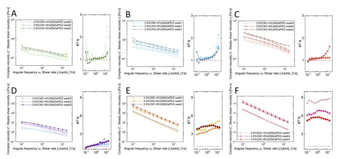
Fig. 4 Time-series Cox-Merz rule rheological analysis: 3.5 wt% CNCs with 4% 20 kDa PEG, 6 wt% 20 kDa PEG and 8% 20 kDa PEG at 0 week (A), 1 week (B) and 4 weeks (C); 4% 200 kDa PEG, 6 wt% 200 kDa PEG and 8 wt% 200 kDa PEG at 0 week (D), 1 week (E) and 4 weeks (F).
