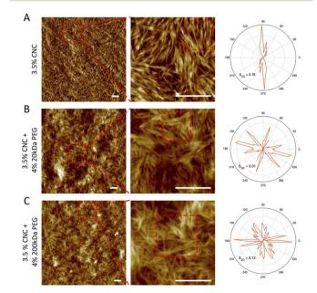
Fig. 6 AFM images and orientation distribution of contour segments within selected areas of pure 3.5 wt% CNCs (A), 3.5 wt% CNCs with 4 wt% 20 kDa PEG (B), 3.5 wt% CNCs with 4 wt% 200 kDa PEG (C) at 1 week. Scale bar: 500 nm.
