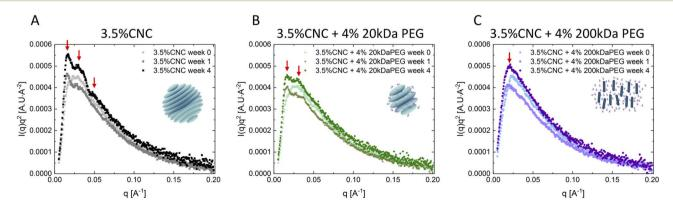
Fig. 5 Time-series Lorentz-corrected scattering intensities as a function of scattering vector q of pure 3.5 wt% CNCs (A), 3.5 wt% CNCs with 4 wt% 20 kDa PEG (B), 3.5 wt% CNCs with 4 wt% 200 kDa PEG (C) at 0 week, 1 week and 4 weeks.
