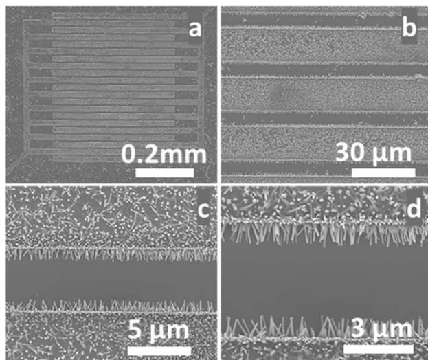
Fig. 6 (a)–(d) SEM images at different magnifications of ZNWs grown on prepatterned Au electrodes on a Si/SiO<sub>2</sub> substrate.
