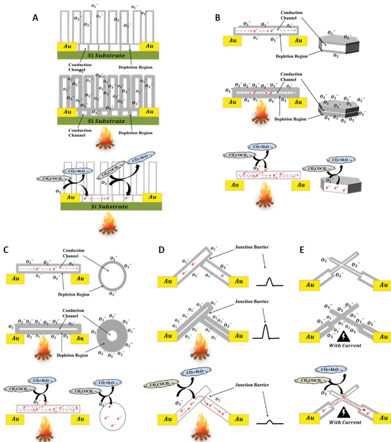
Fig. 9 A schematic diagram explaining the sensing mechanism of the (A) ZNWA GS, (B) ZND GS, (C) SZNW GS, (D) BZNW GS, and BZNN GS.
