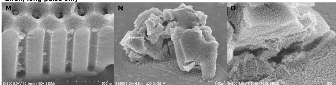
Fig. 2 SEM micrographs of calcined VPI experiments on AAO (first column) and glass (second and third columns) substrates with either one cycle of long pulses or 10 cycles with short pulses. (A–C) Alumina with long pulses. (D–F) Alumina with short pulses. (G–I) Titania with long pulses. (J–L) Titania with short pulses. (M–O) Zinc oxide with long pulses.
