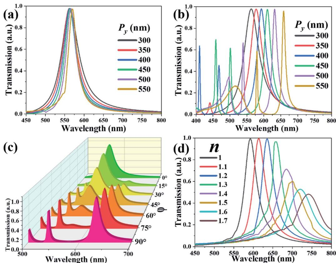
Fig. 6 Transmission spectra of TCF-2 with different  $P_y$  values from 300 nm to 550 nm at normal incidence in (a) TE and (b) TM modes. Transmission spectra of TCF-2 (c) with different  $\varphi$  values at the normal incidence and (d) exposed to the ambient environment with different  $n$  values under the condition of  $P_x = 300$  nm and  $P_y = 500$  nm under normal TE-polarized incident light.
