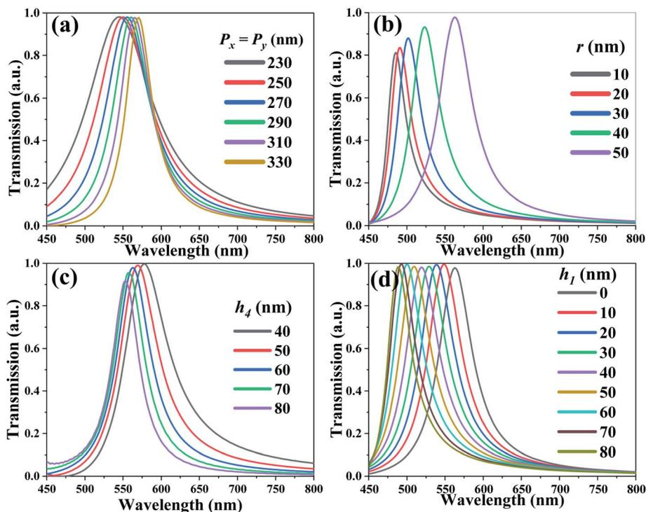
Fig. 2 Transmission spectra of TCF-1 with different values of (a) periods ( $P_x = P_y$ ) from 230 nm to 330 nm, (b)  $r$  from 10 nm to 50 nm, (c) thickness of Ag nanoholes ( $h_3$ ) from 40 nm to 80 nm, and (d)  $h_1$  from 0 nm to 80 nm under normal TE-polarized incident light.
