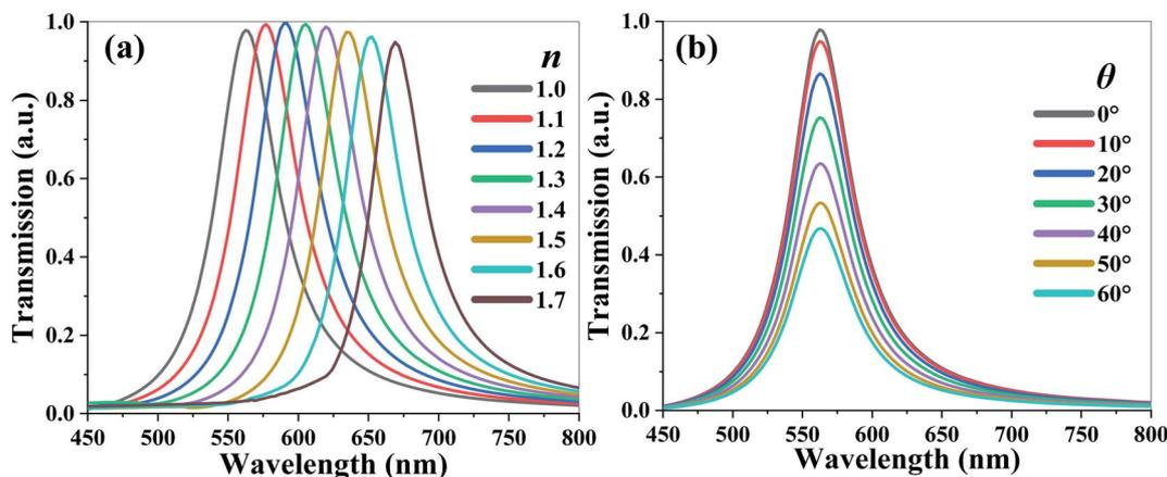
Fig. 3 Transmission spectra of TCF-1 (a) exposed to the ambient environment with different  $n$  values from 1.0 to 1.7 under normal TE-polarized incident light and (b) with different  $\theta$  values from  $0^\circ$  to  $60^\circ$  in TE mode.
