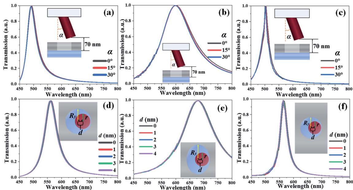
Fig. 7 Transmission spectra of (a) and (d) TCF-1, (b) and (e) TCF-2 and (c) and (f) TCF-3 with different (a–c)  $\alpha$  values and (d–f)  $d$  values while keeping other parameters as constants under normal TE-polarized incident light.
