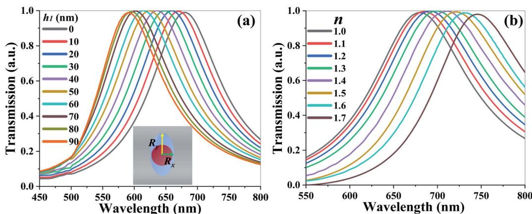
Fig. 5 Transmission spectra of TCF-2 (a) with different  $h_1$  values from 0 nm to 90 nm and (b) exposed to the ambient environment with different  $n$  values from 1.0 to 1.7 under the condition of  $R_x = 60$  nm,  $R_y = 90$  nm under normal TE-polarized incident light.
