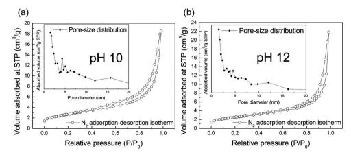
Fig. 6  $N_2$  adsorption—desorption isotherms of the samples synthesized at pH 10 (a) and 12 (b), respectively. The inset is pore-size distribution of the corresponding samples.
