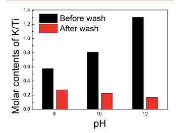
Fig. 3 The molar contents of K/Ti in the powder prepared from the peroxo-titanium complex ion at pH 8, 10, and 12, respectively. Black bars display the data of the samples before wash, and red bars display the data of the samples after wash.
