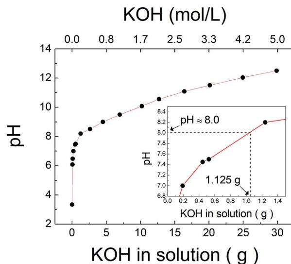
Fig. 2 The variation of pH according to the amount and concentration of  $\text{KOH}$  in solution injected into  $\text{H}_2\text{O}_2$ . The inset enlarged range corresponded to 1.125 g of  $\text{KOH}$ .
