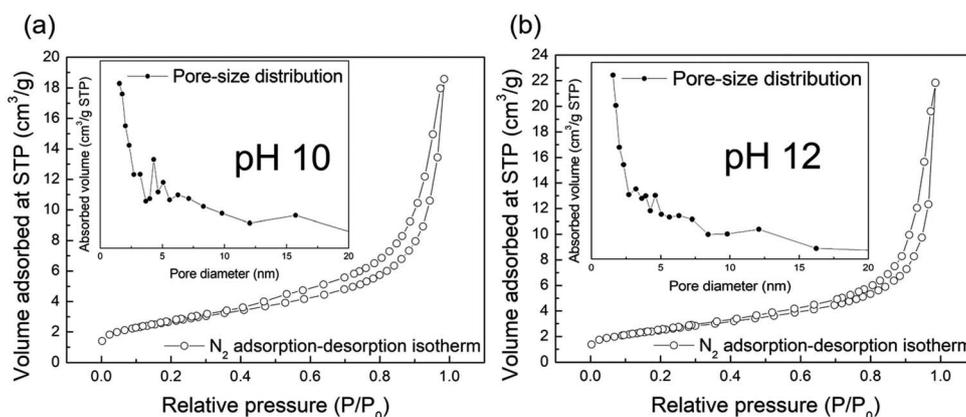
Fig. 6 N<sub>2</sub> adsorption–desorption isotherms of the samples synthesized at pH 10 (a) and 12 (b), respectively. The inset is pore-size distribution of the corresponding samples.
