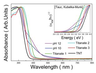
Fig. 7 Absorbance spectra of titanate prepared by various methods. The inset shows Tauc plots to observe the optical band-gap energy corresponding to the samples.
