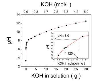
Fig. 2 The variation of pH according to the amount and concentration of KOH in solution injected into  $H_2O_2$ . The inset enlarged range corresponded to 1.125 g of KOH.
