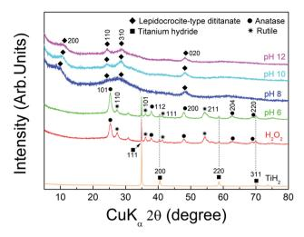
Fig. 1 XRD patterns of powders synthesized from the ionic solution at the conditions of  $H_2O_2$ , pH 6, 8, 10, and 12, respectively, and commercial  $TiH_2$  powder.
