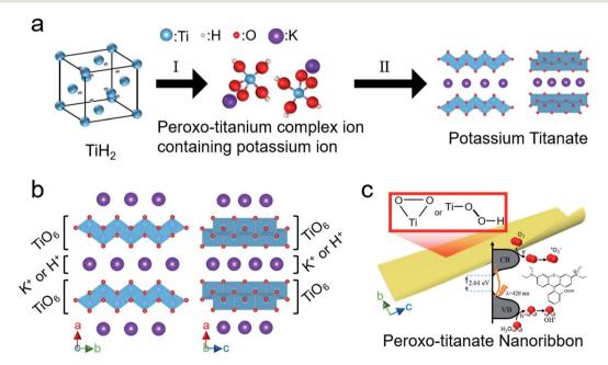
Fig. 10 (a) A schematic of the proposed bottom-up synthesis route for peroxo-titanate nanoribbons; (I) formation of the peroxo-titanium complex ion containing potassium ions from  $TiH_2$  powder by treating with  $H_2O_2/KOH$  solution. (II) Formation of layered titanate from peroxotitanium complex ions. (b) Hypothetical schematic crystal structures along [001] and [010] of hydrogenated potassium titanate. (c) Formation of peroxo-titanate nanoribbons with enhanced photocatalytic activity.
