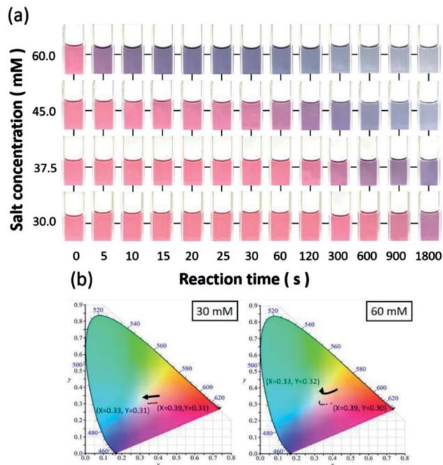
Fig. 4 (a) Visual colorimetric table of  $\text{Na}^+$  ion detection under various salt concentrations and reaction durations. CIE chromaticity diagrams of AuNP probes in the presence of (b) 30 mM (left diagram) and 60 mM (right diagram) of sodium salts.
