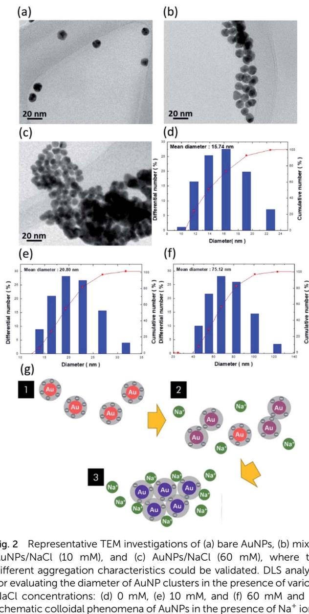
Fig. 2 Representative TEM investigations of (a) bare AuNPs, (b) mixed AuNPs/NaCl (10 mM), and (c) AuNPs/NaCl (60 mM), where the different aggregation characteristics could be validated. DLS analysis for evaluating the diameter of AuNP clusters in the presence of various NaCl concentrations: (d) 0 mM, (e) 10 mM, and (f) 60 mM and (g) schematic colloidal phenomena of AuNPs in the presence of  $\text{Na}^+$  ions.
