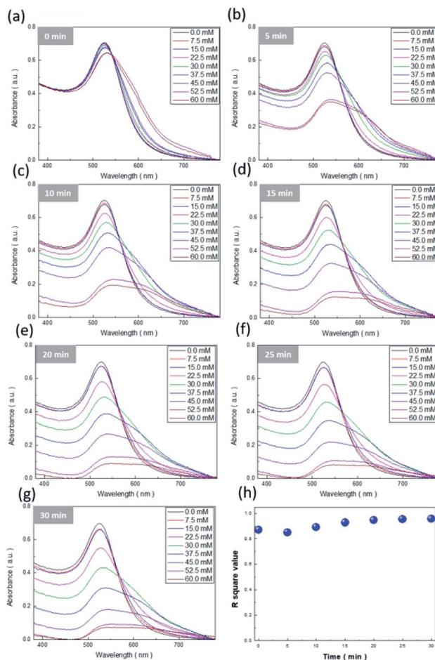
Fig. 8 Colorimetric sensitivity tests of Na<sup>+</sup> ions with various concentrations from 0 to 60 mM under different reaction durations: (a) 0 min, (b) 5 min, (c) 10 min, (d) 15 min, (e) 20 min, (f) 25 min, and (g) 30 min. (h) Correlation of  $R^2$  values extracted from the linear regression of the measured results presented in (a–g), with respect to various reaction durations.
