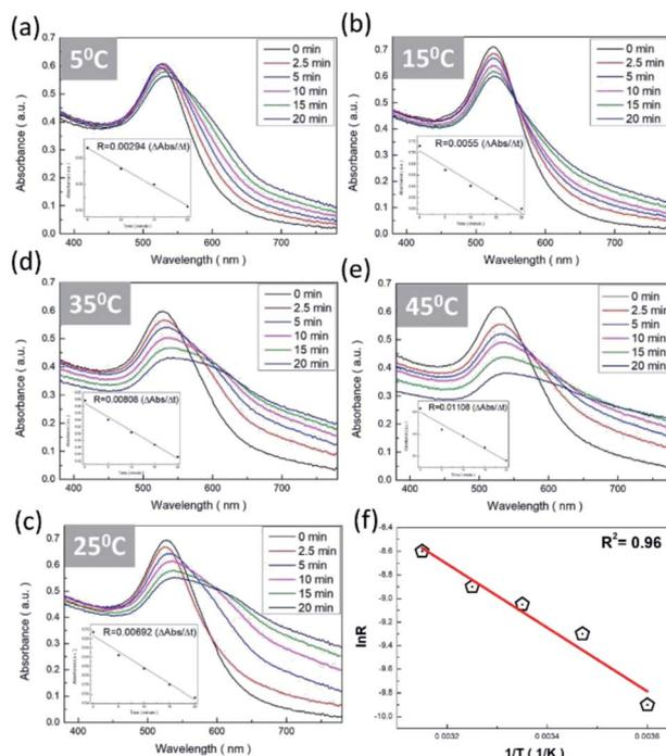
Fig. 7 Colorimetric sensitivity tests of  $\text{Na}^+$  ions under various environmental temperatures: (a)  $5^\circ\text{C}$ , (b)  $15^\circ\text{C}$ , (c)  $25^\circ\text{C}$ , (d)  $35^\circ\text{C}$ , and (e)  $45^\circ\text{C}$ . (f) Correlation of rate constants in natural logarithm form and corresponding inverse temperatures. The linear regression possessed the  $R^2$  of 0.96.
