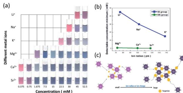
Fig. 5 (a) Comparative colorimetric examinations of AuNP probes for detecting various cation ions. (b) Plot of the detectable minimum concentration of various cation ions with respect to the corresponding ion radiuses. (c) Illustrated detection mechanism of AuNP probes influenced by ion radius and charge of target analytes.
