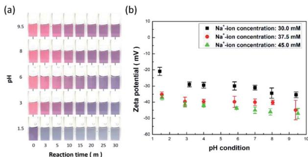
Fig. 6 (a) Colorimetric examinations of  $\text{Na}^+$  ions under various pH conditions. (b) Measured zeta potentials of analyte solutions in the presence of  $\text{Na}^+$  ions with concentrations of 30.0, 37.5, and 45.0 mM under different pH values.
