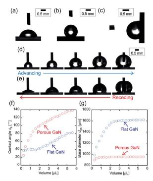
Fig. 3 Optical micrographs of water droplets on (a) flat GaN, (b) porous GaN, and (c) porous GaN at a 90° tilt angle. (d and e) Optical micrographs of a water droplet on porous GaN when the water droplet is inflated and deflated, respectively. (f and g) Receding contact angle and base diameter of flat and porous GaN *versus* the volume of the water droplet, respectively.
