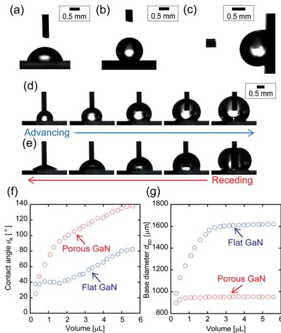
Fig. 3 Optical micrographs of water droplets on (a) flat GaN, (b) porous GaN, and (c) porous GaN at a  $90^\circ$  tilt angle. (d and e) Optical micrographs of a water droplet on porous GaN when the water droplet is inflated and deflated, respectively. (f and g) Receding contact angle and base diameter of flat and porous GaN versus the volume of the water droplet, respectively.
