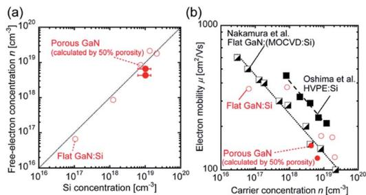
Fig. 2 Comparison of the electrical properties of porous and flat GaN. (a) Relationship between the Si concentration and net donor concentration for porous and flat GaN grown by HF-VPE. (b) Dependence of electron mobility on carrier concentration for GaN layers at 300 K.
