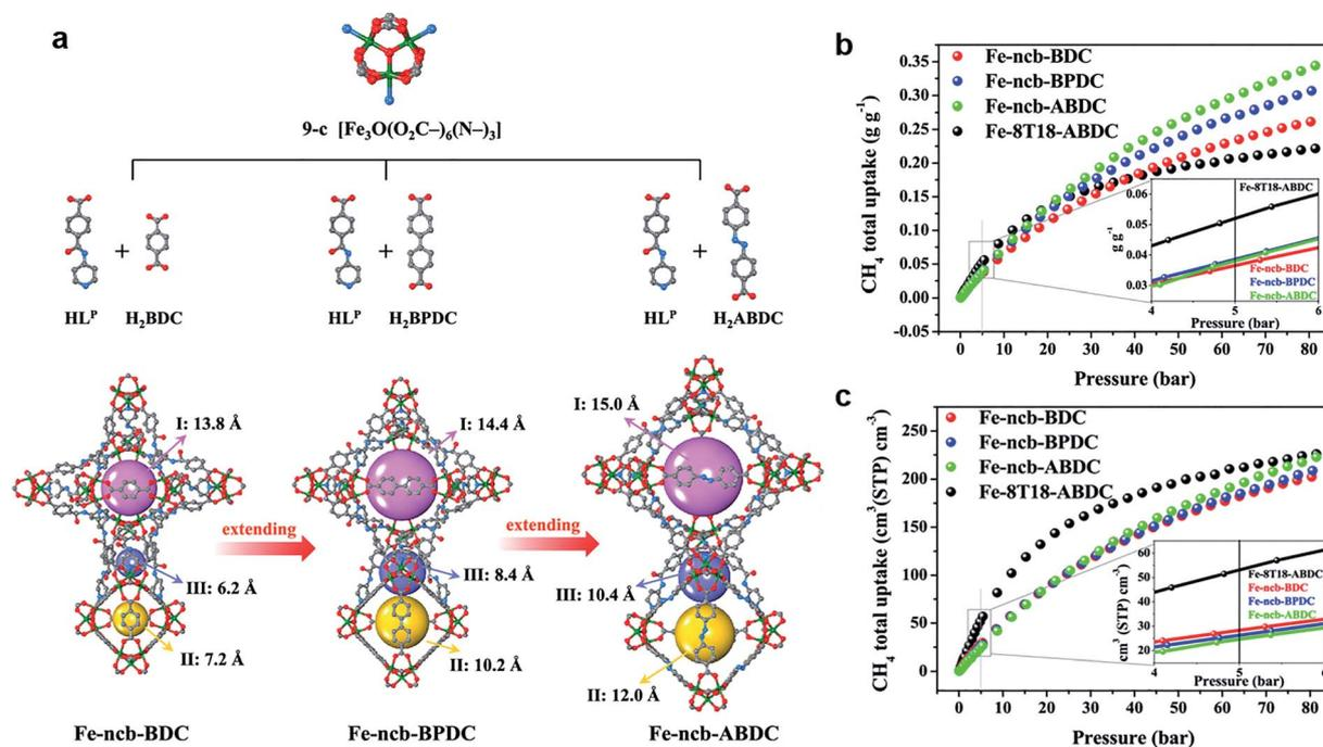
Fig. 5 (a) The constructions of Fe-ncb-MOFs. (b) The  $\text{CH}_4$  gravimetric adsorption isotherms at 298 K. (c) Volumetric adsorption isotherms at 298 K.<sup>51</sup> Reproduced from ref. 51 with permission, copyright The American Chemical Society, 2021.
