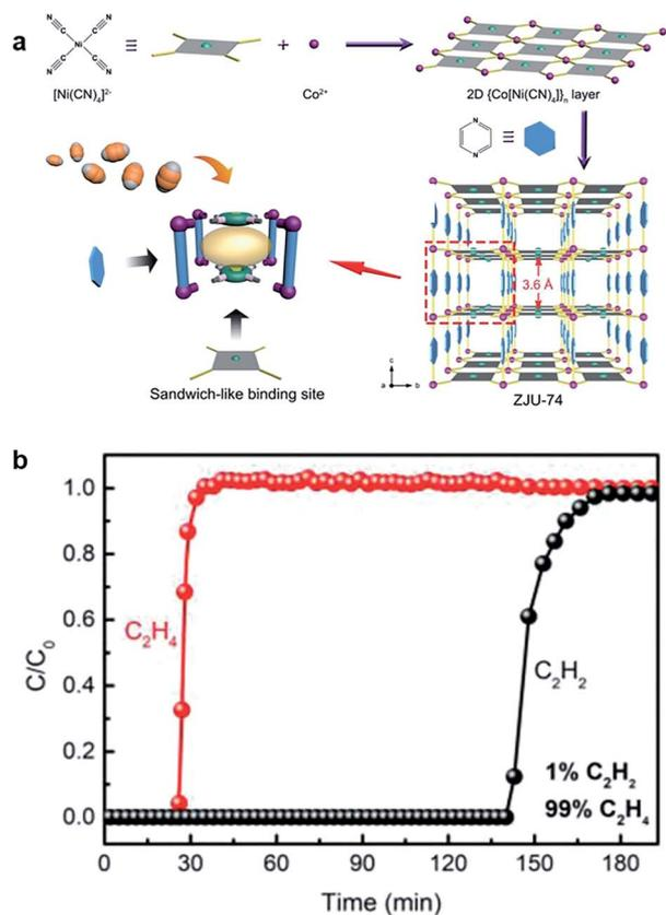
Fig. 8 (a) The construction process of ZJU-74a, 3D framework, and sandwich-like binding sites. (b) Experimental column breakthrough curves for a 1/99  $C_2H_2/C_2H_4$  mixture at 298 K and 1 bar.<sup>68</sup> Reproduced from ref. 68 with permission, copyright John Wiley and Sons, 2020.
