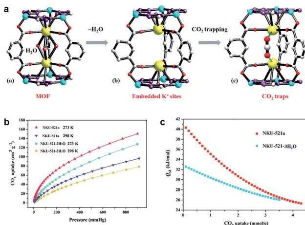
Fig. 2 (a) The structure of NKU-521, NKU-521a, and NKU-521a· $\text{CO}_2$  (according to the molecular simulation), (b) the  $\text{CO}_2$  adsorption isotherms, (c)  $Q_{st}$  toward  $\text{CO}_2$  for NKU-521-3H<sub>2</sub>O and NKU-521a at 273 K and 298 K.<sup>39</sup> Reproduced from ref. 39 with permission, copyright John Wiley and Sons, 2019.
