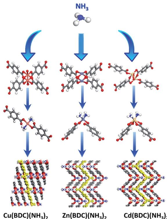
Fig. 4 The transform of  $\text{M}(\text{BDC})$  ( $\text{M} = \text{Cu}, \text{Zn}, \text{Cd}$ ).<sup>42</sup> Reproduced from ref. 42 with permission, copyright American Chemical Society, 2020.
