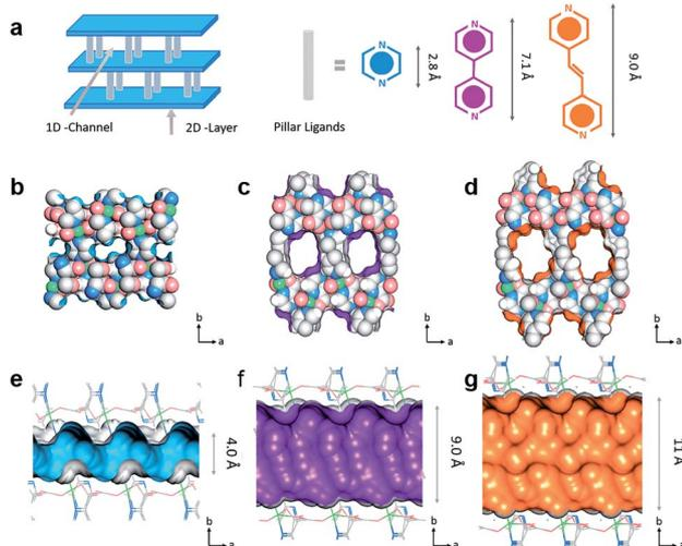
Fig. 7 (a) The crystal structure of  $[Cu_2(pzdc)_2L]$ . The pore constructed by three ligands of (b) and (e) CPL-1, (c) and (f) CPL-2, (d) and (g) CPL-5.<sup>67</sup> Reproduced from ref. 67 with permission, copyright The American Chemical Society, 2019.
