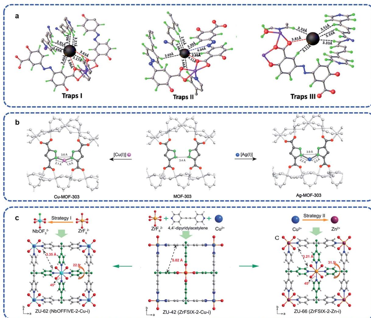
Fig. 13 (a) Three adsorption traps in ECUT-60.<sup>82</sup> Reproduced from ref. 82 with permission, copyright Elsevier, 2021. (b) The chelated structure of Cu-MOF-303 and Ag-MOF-303 derived from MOF-303.<sup>62</sup> Reproduced from ref. 62 with permission, copyright John Wiley and Sons, 2020. (c) The interpenetrated networks of ZU-62, ZU-42, and ZU-66 (viewed along the *c*-axis).<sup>84</sup> Reproduced from ref. 84 with permission, copyright John Wiley and Sons, 2020.
