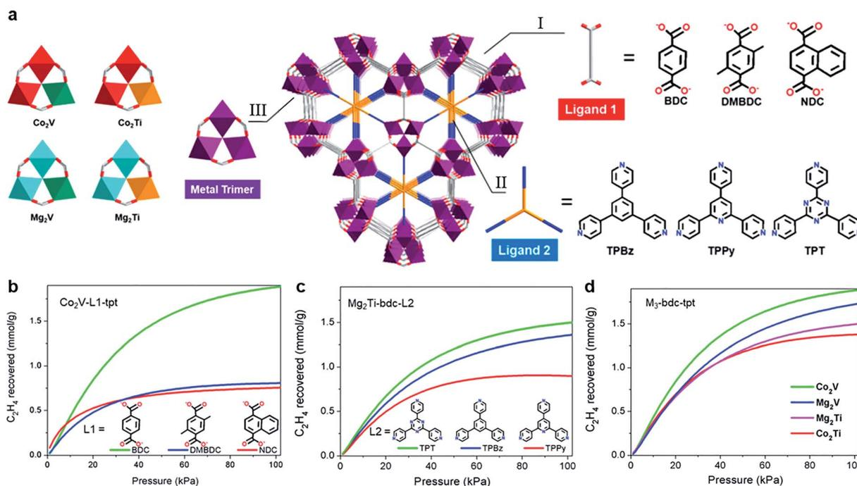
**Fig. 11** (a) The frameworks composed by three kinds of ligand 1, three kinds of ligand 2, and four kinds of metal cluster. (b) Contradistinction of C<sub>2</sub>H<sub>6</sub>/C<sub>2</sub>H<sub>4</sub> (50/50) separation potential of Co<sub>2</sub>V-L1-tpt, (c) Mg<sub>2</sub>Ti-bdc-L<sub>2</sub>, and (d) M<sub>3</sub>-bdc-tpt.<sup>76</sup> Reproduced from ref. 76 with permission, copyright The American Chemical Society, 2020.
