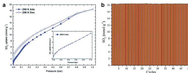
Fig. 3 (a) The  $\text{SO}_2$  adsorption–desorption isotherm of MIL-101(Cr)-4F(1%), illustration: adsorption isotherm enlarged from 0.0–0.1 bar. (b) Adsorption–desorption cycles for 101(Cr)-4F(1%) at 298 K and 1 bar.<sup>40</sup> Reproduced from ref. 40 with permission, copyright The Royal Society of Chemistry, 2020.
