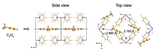
Fig. 9 Schematic diagram of GeFSIX-dps-Cu after adsorbing  $C_3H_4$ .<sup>69</sup> Reproduced from ref. 69 with permission, copyright John Wiley and Sons, 2020.
