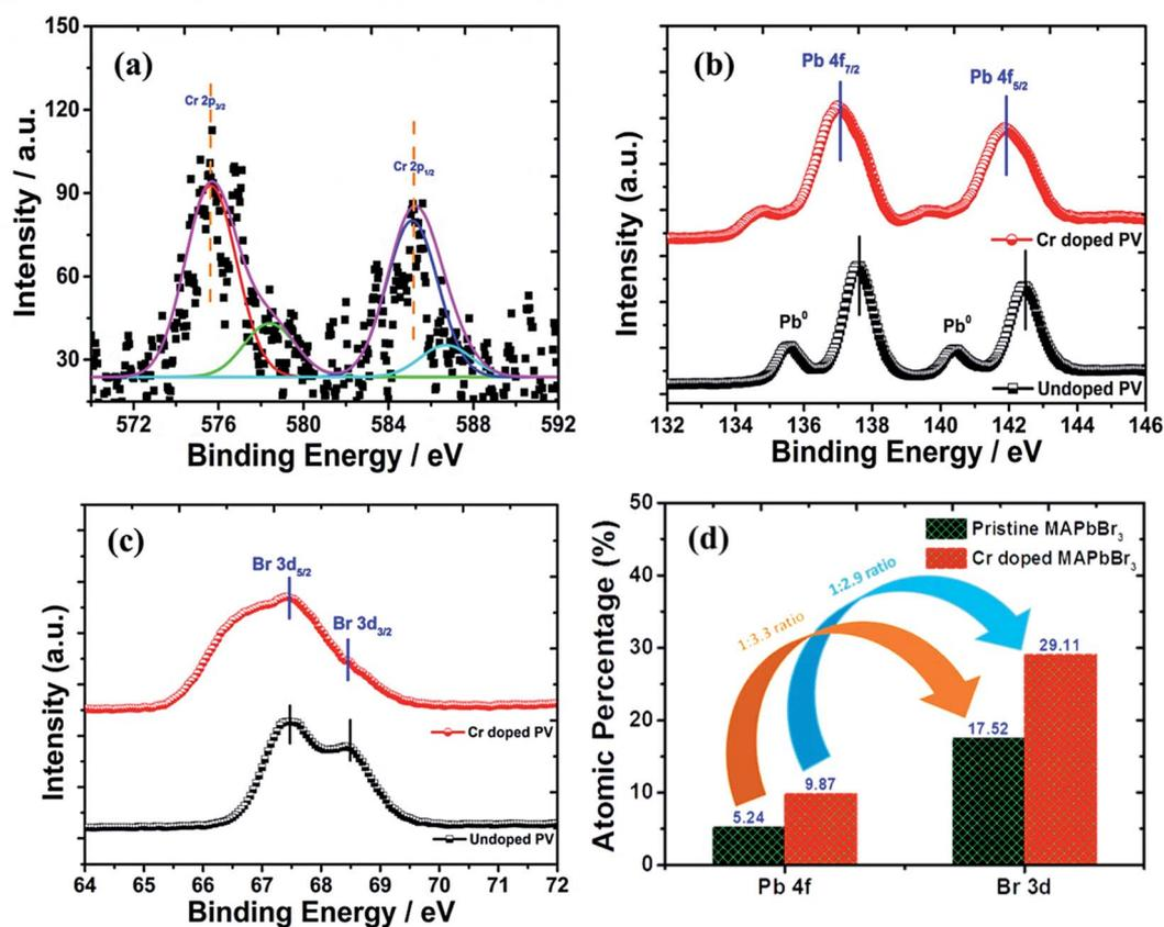
Fig. 6 XPS spectral plots of (a) Cr 2p spectrum, (b) Pb 4f spectra, (c) Br 3d spectrum and (d) histogram profile of the relative change in Pb : Br ratios of Cr-doped perovskite nanocrystals.
