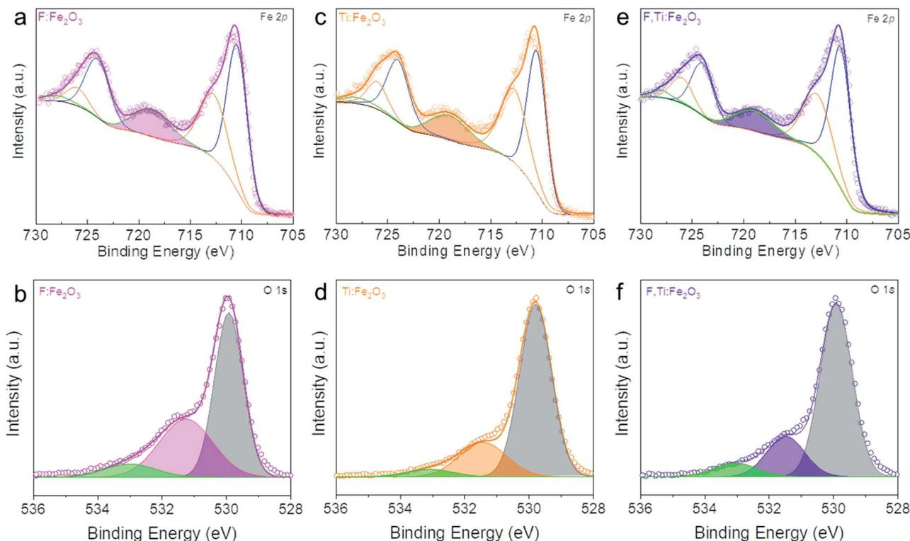
Fig. 4 Fe 2p and O 1s XPS spectra of F:Fe<sub>2</sub>O<sub>3</sub> (a) and (b), Ti:Fe<sub>2</sub>O<sub>3</sub> (c) and (d) and F,Ti:Fe<sub>2</sub>O<sub>3</sub> (e) and (f). The coloured peaks in (a), (c), and (e) denote the Fe<sup>3+</sup> satellite peak. Core-level O 1s XPS spectra in (b), (d), and (f) show the Fe–O bond, oxygen vacancy, and surface hydroxyl group peaks, respectively, from low to high binding energies.
