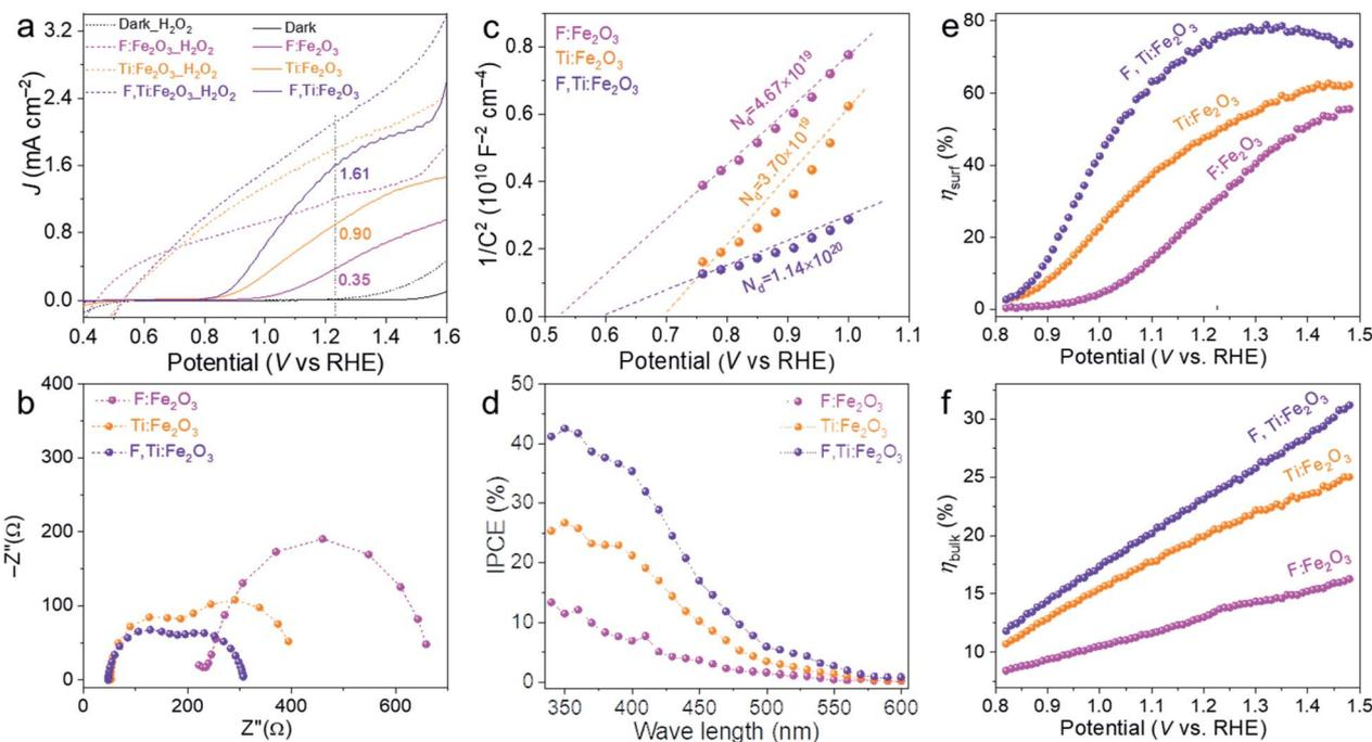
Fig. 6 *J*-*V* curves with (dashed) and without (solid) the H<sub>2</sub>O<sub>2</sub> hole scavenger in electrolyte (a), Nyquist plots (b), Mott-Schottky plots (c), IPCE (d),  $\eta_{\text{surf}}$  (e) and  $\eta_{\text{bulk}}$  (f) of F:Fe<sub>2</sub>O<sub>3</sub>, Ti:Fe<sub>2</sub>O<sub>3</sub>, and F,Ti:Fe<sub>2</sub>O<sub>3</sub>. The PEC water oxidation was performed under 1 sun irradiation (100 mW cm<sup>-2</sup>) in 1 M NaOH electrolyte.
