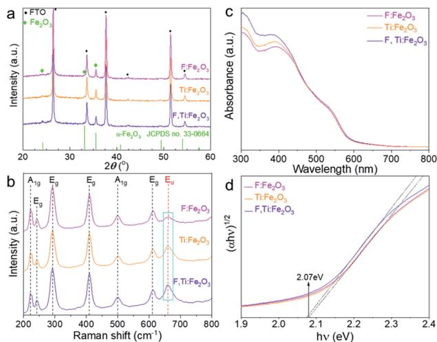
Fig. 3 XRD patterns (a), Raman spectra (b), light absorption spectra (c) and Tauc plots (d) of Fe<sub>2</sub>O<sub>3</sub>, F:Fe<sub>2</sub>O<sub>3</sub>, Ti:Fe<sub>2</sub>O<sub>3</sub>, and F,Ti:Fe<sub>2</sub>O<sub>3</sub> photoanodes.
