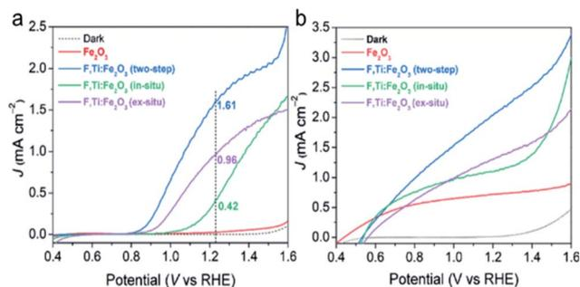
Fig. 5 Comparison of single-step (*in situ* or *ex situ*) and two-step (*in situ* followed by *ex situ*) co-doping of F and Ti into hematite to fabricate the F,Ti:Fe<sub>2</sub>O<sub>3</sub> photoanode. (a) *J*-*V* curves of water oxidation (without H<sub>2</sub>O<sub>2</sub>). (b) *J*-*V* curves of H<sub>2</sub>O<sub>2</sub> oxidation. The PEC water oxidation was performed under 1 sun irradiation (100 mW cm<sup>-2</sup>) in 1 M NaOH electrolyte.
