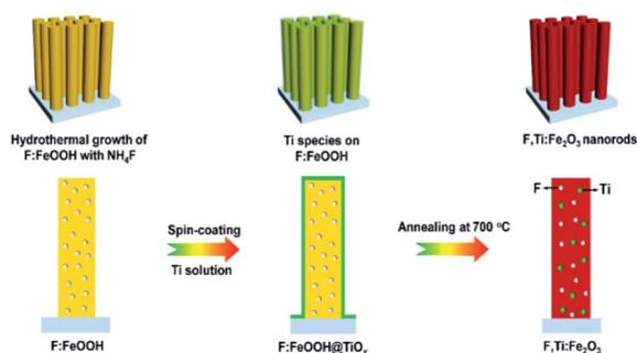
Fig. 1 Schematic synthesis procedure of F,Ti:Fe<sub>2</sub>O<sub>3</sub> nanorods via the two-step co-doping process of *in situ* F-doping and *ex situ* external Ti-doping.
