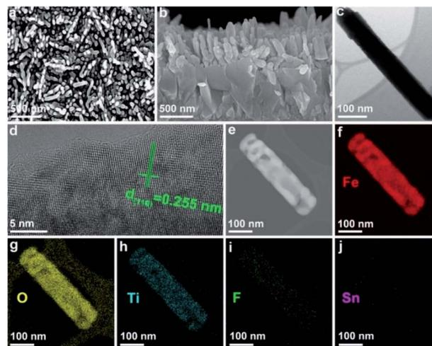
Fig. 2 SEM (top view (a) and cross-sectional (b)), TEM (c), HRTEM (d), HAADF (e), and elemental mapping images of Fe (f), O (g), Ti (h), F (i), and Sn (j) of F,Ti:Fe<sub>2</sub>O<sub>3</sub> nanorods.
