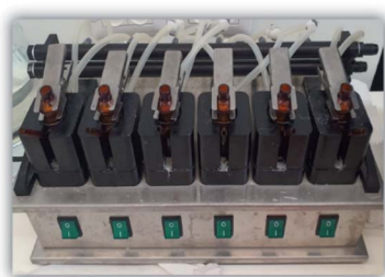
Scheme 1 Efficacy experiments with a Franz diffusion cell apparatus (PermeGear, PA, USA).
