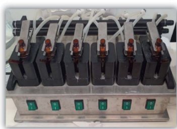
Scheme 1 Efficacy experiments with a Franz diffusion cell apparatus (PermeGear, PA, USA).
