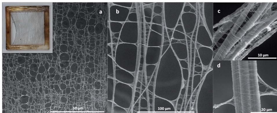
Fig. 3 (a–d) SEM images of the silver NW coated PLGA fabric-like substrate formed of thin fibres (1–2  $\mu\text{m}$ ). Inset: an image of the silver NW coated PLGA fabric-like substrate glued to a PET frame.
