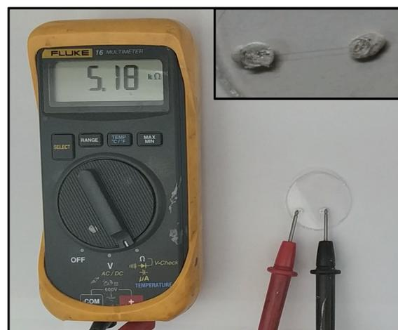
**Fig. 2** Resistance measurement of a single PLGA fibre of  $20\ \mu\text{m}$  in diameter and  $\sim 1\ \text{cm}$  in length. The  $5.18\ \text{k}\Omega$  resistance is translated to a sheet resistance of  $32\ \Omega\ \text{sq}^{-1}$  using the dimensions of the fibre. The inset shows a zoom-in view of the silver-paint contacted fibre.
