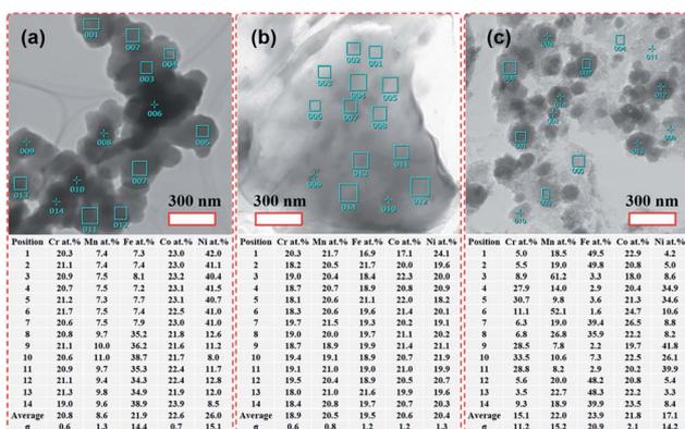
Fig. 3 TEM images of the HEH-1# as-synthesized products under various synthesis conditions and corresponding chemical compositions. (a) EG-K. (b) EG-K/N. (c) H<sub>2</sub>O-K/N.
