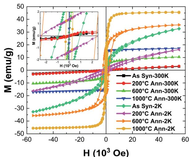
Fig. 10 Magnetization curves vs. magnetic field ( $M$ – $H$  curves) for HEH-1# EG-K/N as-synthesized and annealed nanoparticles recorded at 300 K and 2 K. The inset shows the expanded view of the  $M$ – $H$  curves.
