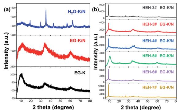
Fig. 1 (a) XRD patterns of the HEH-1# as-synthesized products under H<sub>2</sub>O-K/N, EG-K/N, and EG-K synthesis conditions. (b) XRD patterns of HEH-2#–7# as-synthesized products under EG-K/N conditions. All samples were synthesized by solvothermal treatment at 200 °C for 2 h.
