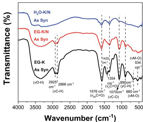
Fig. 5 FT-IR spectra of the HEH-1# as-synthesized products under EG-K, EG-K/N, and H<sub>2</sub>O-K/N conditions.
