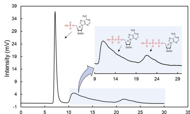
Fig. 6 Chromatogram of nucleotides with a meter-long ZnO-NW column with the phosphate gradient condition. LC conditions: column, ZnO-NWs (90 cm  $\times$  100  $\mu\text{m}$ ); mobile phase, A: water, B: 250 mM phosphate buffer; gradient condition, 0–1 min, 100% A, 1–21 min 0% B to 100% B, 21–30 min 100% B; flow rate, 1.0  $\mu\text{L min}^{-1}$ ; temperature 25  $^{\circ}\text{C}$ ; detection, UV (260 nm).
