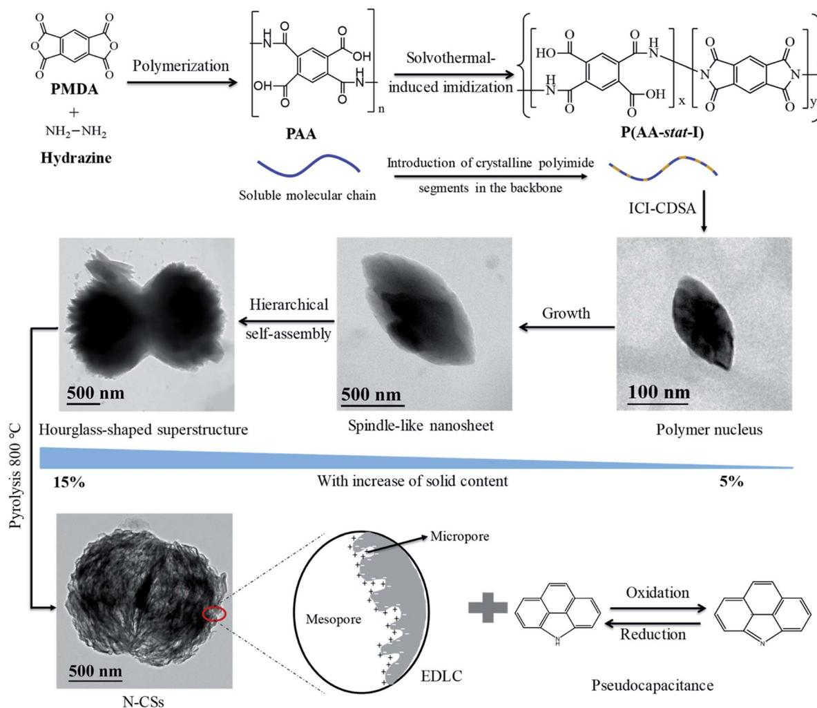
**Scheme 1** Synthesis of PAA *via* stepwise polymerization and the corresponding thermally induced imidization reaction. With the formation of polyimide segments, spindle-like nanosheets were formed by ICI-CDSA, which further self-assembled to an hourglass-shaped nanostructure at high concentration. The N-CSs with multi-level pores could be obtained by the pyrolysis of the hourglass-shaped precursors at 800 °C. And the schematic illustration of the EDLC and pseudocapacitance of N-CSs.
