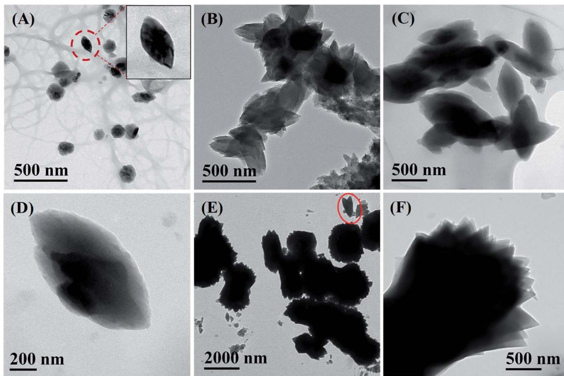
Fig. 2 Monitoring the formation process of the hourglass-shaped superstructures at different concentrations in DMF by TEM. (A) 50, (B) 75, (C and D) 100 and (E and F) 125 mg mL<sup>-1</sup>. The nanosheets in the red circle in (E) are spindle-like nanosheets.
