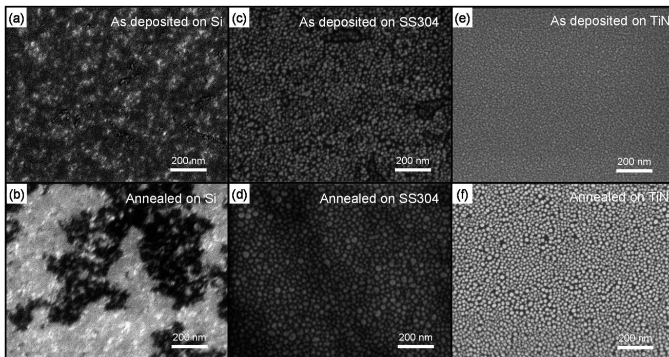
Fig. 1 Top-view high-resolution SEM images of the as-deposited and annealed Au on Si (a, b), SS304 (c, d), and TiN (e, f).
