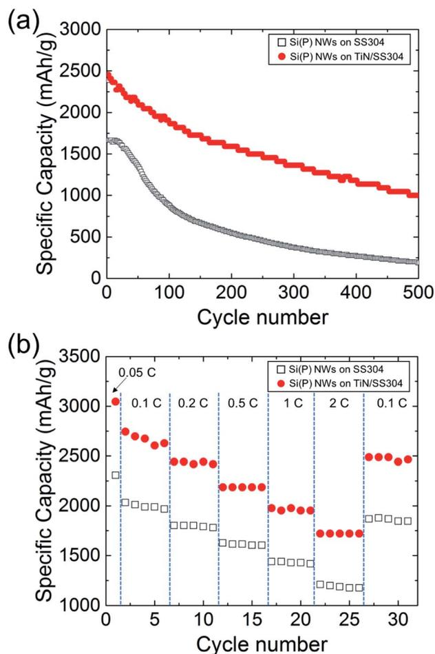
Fig. 5 Specific gravimetric capacities of Si(P) NWs grown on SS304 (black, square, empty) and on TiN/SS304 (red, circle, solid) over cycling at 800 mA g<sup>-1</sup> (0.2C for Si) (a) and at different charging rates (b).
