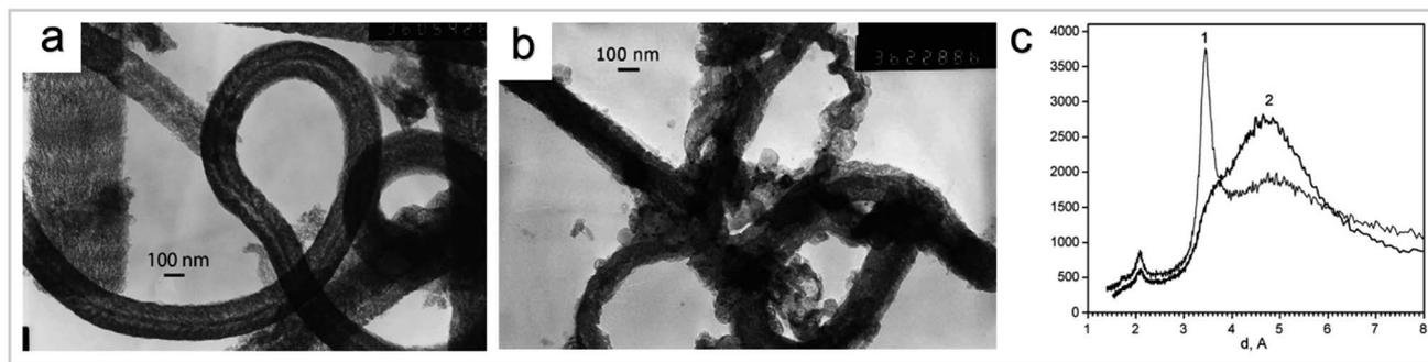
Fig. 7 (a) Typical electron image of CNF obtained by a CVD method from acetylene on the Fe/C/SiO<sub>2</sub> catalyst. (b) Typical electron image of CNF activated with melted KOH modified with 2 wt% of copper. (c) XRD patterns of CNF (curve 1) and CNF activated with melted KOH (curve 2) "reproduced from ref. 34 with permission from Elsevier, copyright 2008".
