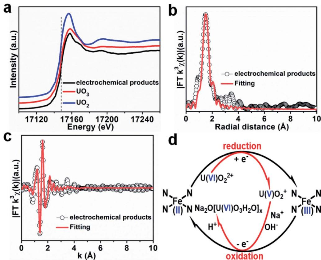
Fig. 15 (a) U L<sub>III</sub>-edge XANES spectra of products using Fe–N<sub>x</sub>–C–R as the catalyst. (b and c) FT-EXAFS spectra and corresponding *R*-space and *k*-space fitting curves of the products. (d) Plausible reaction mechanism for the Fe–N<sub>x</sub>–C–R catalyzed extraction of U(vi) from seawater “reproduced from ref. 82 with permission from Wiley, copyright 2021”.
