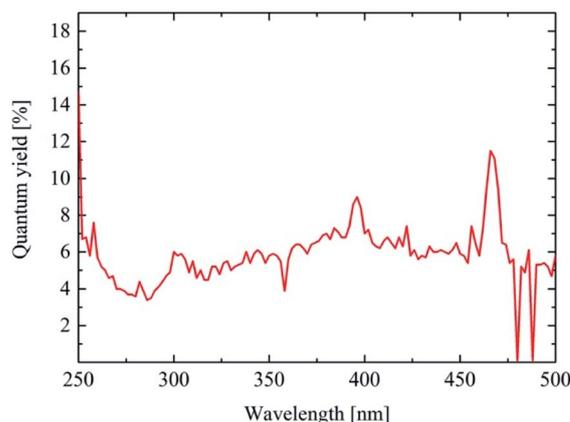
Fig. 5 Photoluminescence quantum efficiency of the as-synthesized  $\text{Y}_2\text{O}_3:\text{Eu}$  nanodiscs at 607 nm as a function of the excitation wavelength. The maximum (approximately 15%) was found near 250 nm. Other maximums (9%) were found at 393 nm (direct  $\text{Eu}^{3+}$  excitation) and 470 nm (12%).
