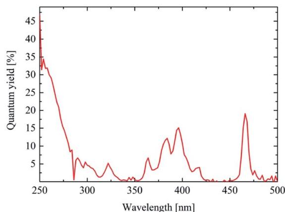
Fig. 7 Photoluminescence quantum efficiency of the annealed (600 °C)  $\text{Y}_2\text{O}_3:\text{Eu}$  nanodiscs at 607 nm as a function of the excitation wavelength. The maximum (>30%) was found near 250 nm. Other maximums (18%) were found at 393 nm (direct  $\text{Eu}^{3+}$  excitation) and 470 nm (20%).
