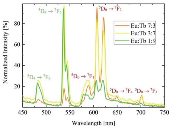
Fig. 4 PL spectra and photographs of the co-doped  $\text{Y}_2\text{O}_3:\text{Eu}$  nanodiscs with different  $\text{Eu} : \text{Tb}$  ratios excited at 273 nm. The red line shows the emission of a  $\text{Eu} : \text{Tb}$  ratio of 7% : 3%, the yellow line 3% : 7% and the green line 1% : 9% ratio. Increasing the Tb concentration results in higher intensities of the characteristic Tb lines at 480 nm and 535 nm. The photographs show the optical colour tunability of the nanomaterial.
