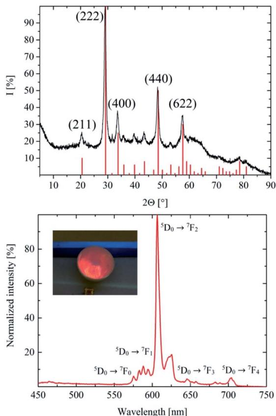
Fig. 6 X-ray diffraction and PL spectrum of the 600 °C annealed  $\text{Y}_2\text{O}_3:\text{Eu}$  10% material. The XRD shows higher crystallinity and no anisotropy in crystal growth when compared to the results obtained from the as-prepared material. Additionally, the PL spectrum matches the characteristic emission spectrum of (bulk)  $\text{Y}_2\text{O}_3:\text{Eu}$ . Inset: a photo of a powder sample, which shows bright red emission under UV excitation.
