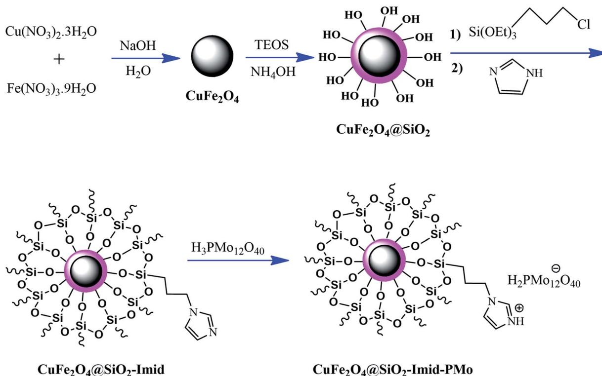
Fig. 13 Synthesis of  $\text{CuFe}_2\text{O}_4@\text{SiO}_2\text{-Imid-PMo}$  catalyst. This figure was adapted with permission from: *Quarterly Journal of Iranian Chemical Communication*, 2019, 7, 271–282.<sup>99</sup>
