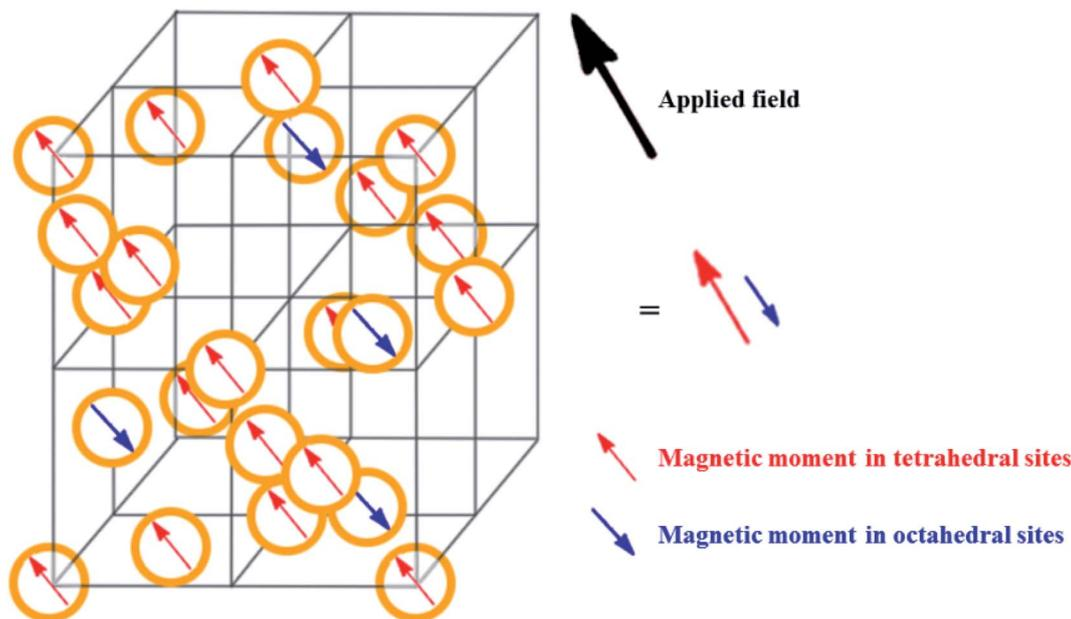
Fig. 39 Spinel structure of ferrites, tetrahedral and octahedral. This figure was adapted with permission from *Int. J. Mol. Sci.*, 2013, 14, 15977–16009.<sup>230</sup>
