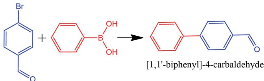
Fig. 4 Suzuki cross-coupling reaction with Pd-Fe<sub>3</sub>O<sub>4</sub>/RGO heterogeneous catalyst. This figure was adapted with permission from H. A. Elazab, 2019 (DOI: 10.9767/bcrec.14.3.3518.478-489).<sup>50</sup>
