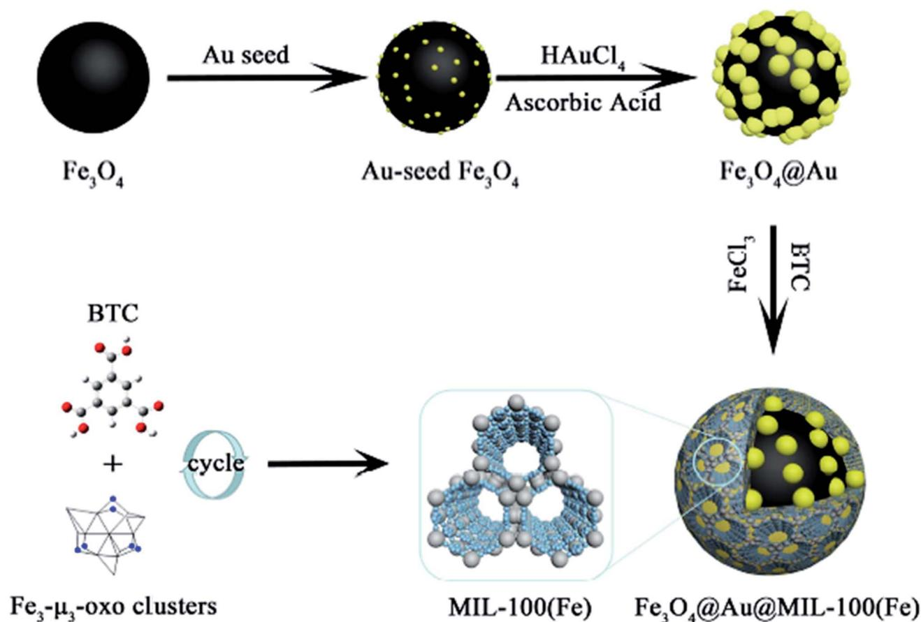
Fig. 10 Illustration of the synthetic route to obtain magnetic MOF-based nanocatalysts. This figure was adapted with permission from ACS Applied Materials & Interfaces, 2018, 10, 25726–25736.<sup>85</sup>
