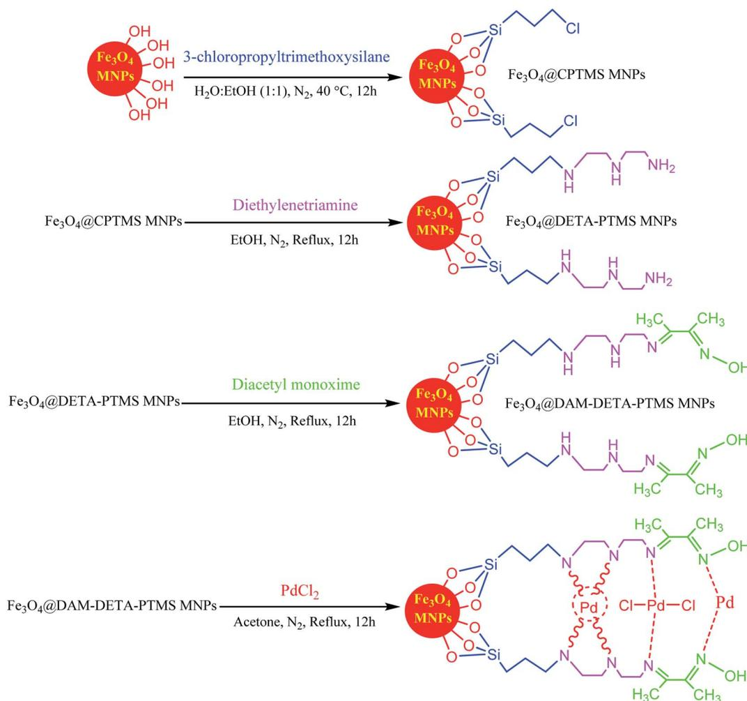
Fig. 1 Synthesis and structure of  $\text{Fe}_3\text{O}_4@\text{Pd-Schiff-base}$  MNPs. This figure was adapted with permission from *Journal of Organometallic Chemistry*, 2019, **880**, 196–212.<sup>49</sup>
