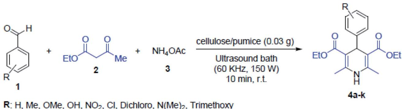
Fig. 31 Synthetic pathway for 1,4-dihydropyridine derivatives using cellulose/pumice nanocomposite catalyst via sonication at room temperature (r.t.). This figure was adapted with permission from *Solid State Sciences*, 2020, 101, 106141.<sup>189</sup>
