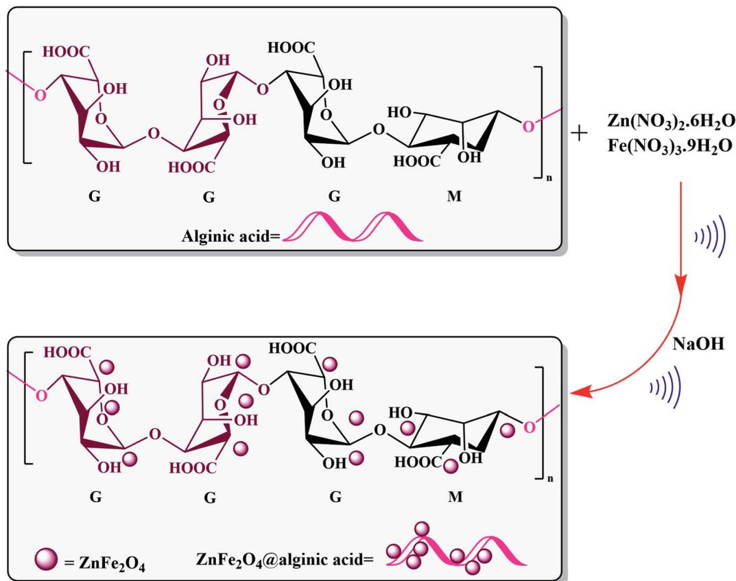
Fig. 8 Synthesis of ZnFe<sub>2</sub>O<sub>4</sub>@alginate. This figure was adapted with permission from *Polyhedron*, 2019, **171**, 193–202.<sup>75</sup>
