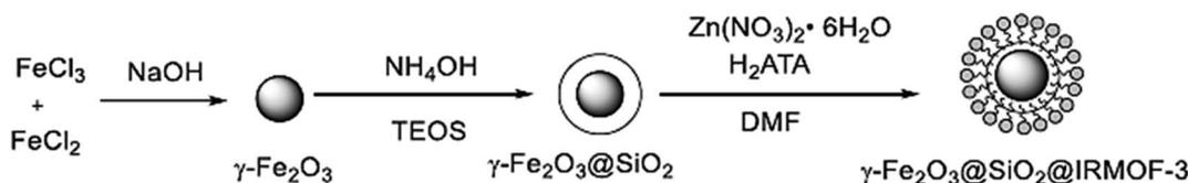
Fig. 29 Schematic showing the preparation of the  $\gamma\text{-Fe}_2\text{O}_3$ @ $\text{SiO}_2$ /IRMOF-3 catalyst. This figure was adapted with a permission from *Journal of Catalysis*, 2020, 387, 39–46.<sup>188</sup>
