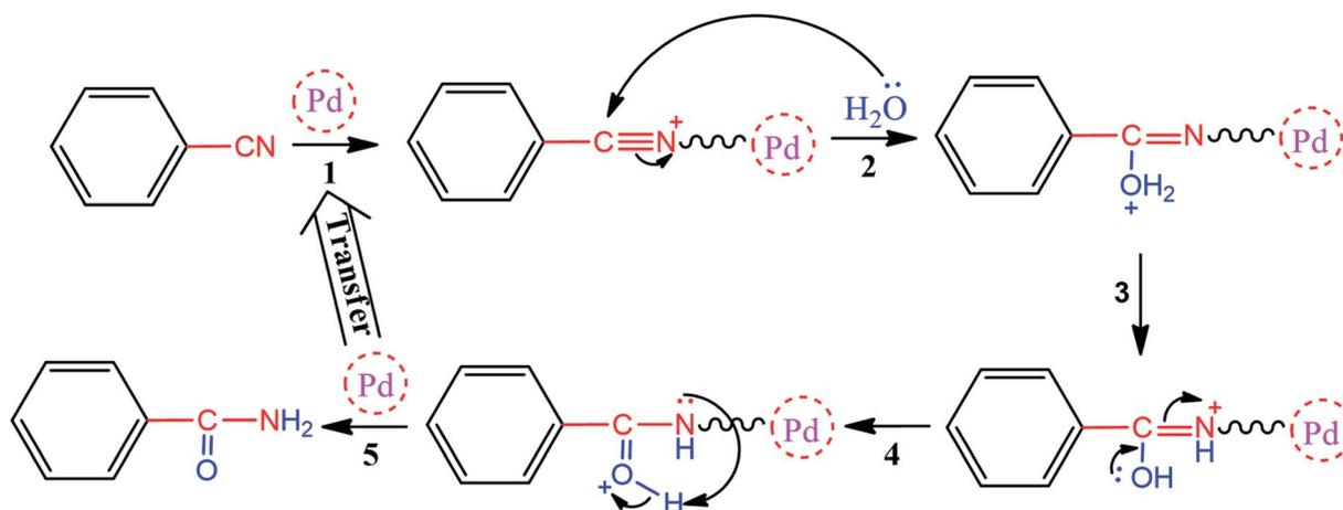
Fig. 3 Proposed mechanism for the synthesis of benzamide. This figure was adapted by permission from *Journal of Organometallic Chemistry*, 2019, **880**, 196–212.<sup>49</sup>
