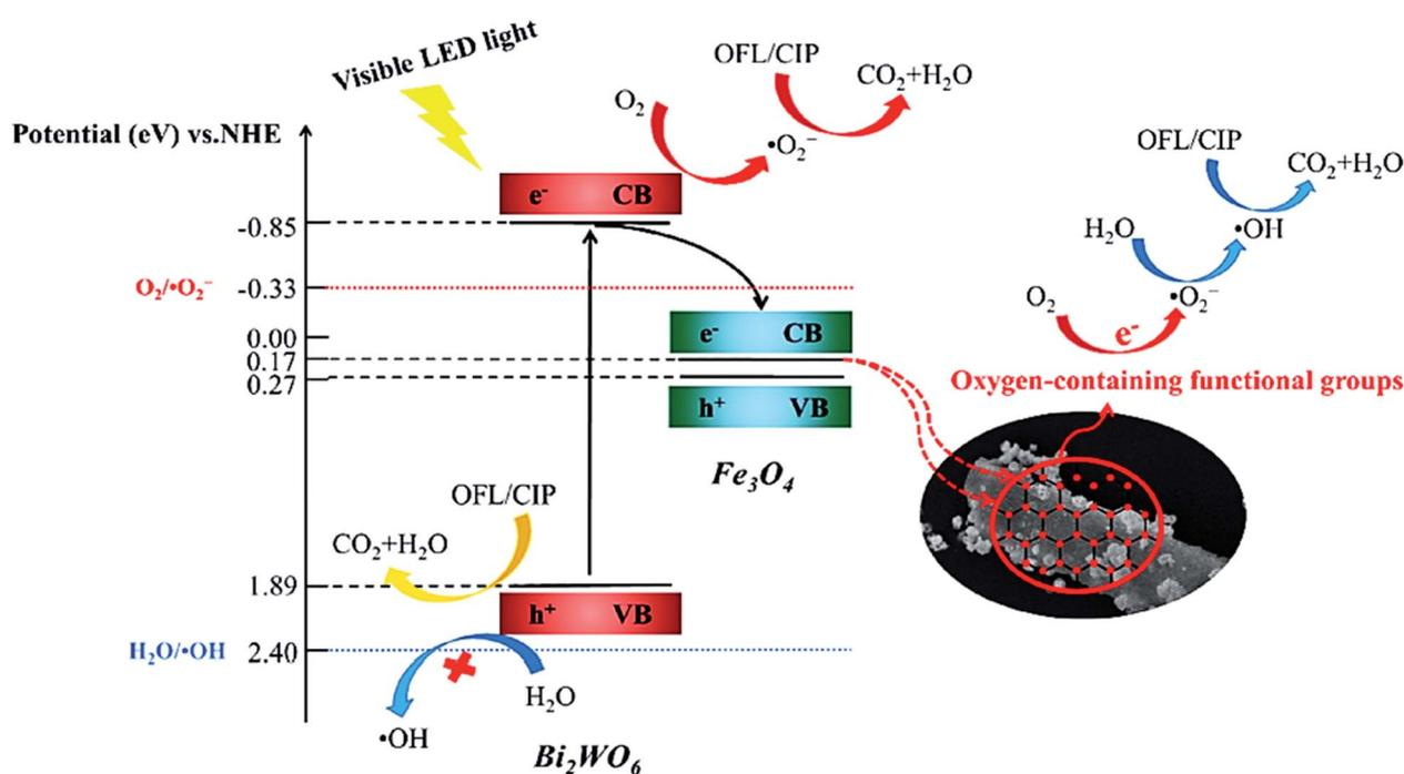
Fig. 26 Plausible mechanism for photocatalytic degradation of OFL and CIP by  $\text{Bi}_2\text{WO}_6/\text{Fe}_3\text{O}_4/\text{BC}$  under visible LED light irradiation. This figure was adapted with permission from *Science of The Total Environment*, 2021, 764, 142879.<sup>161</sup>
