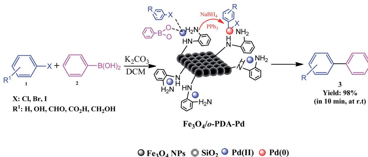
Fig. 27 Schematic of Suzuki–Miyaura cross-coupling reaction conducted using magnetic  $\text{Fe}_3\text{O}_4/o\text{-PDA-Pd}$  nanocatalyst at room temperature (r.t). This figure was adapted with permission from *Journal of Physics and Chemistry of Solids*, 2020, **136**, 109200.<sup>17</sup>
