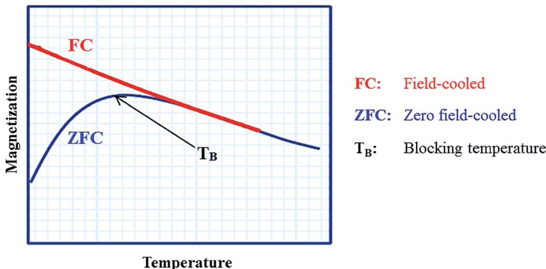
Fig. 37 Effect of temperature. This figure was adapted with permission from *Int. J. Mol. Sci.*, 2013, 14, 15977–16009.<sup>230</sup>
