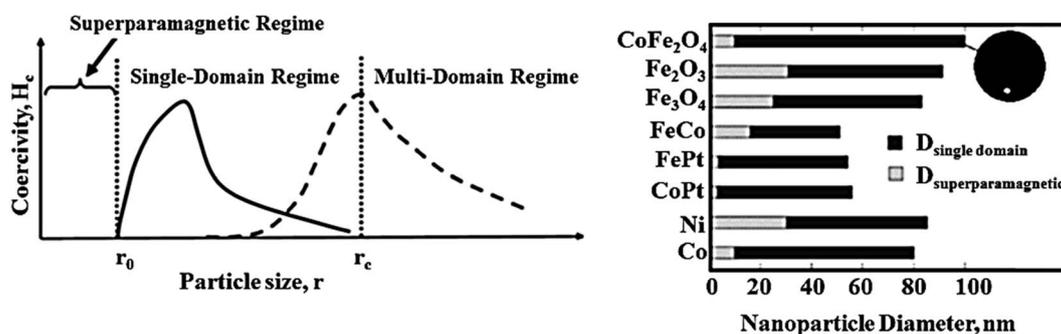
Fig. 38 Particle size and its effect on magnetization. This figure was adapted with permission from *Int. J. Mol. Sci.*, 2013, 14, 15977–16009.<sup>230</sup>
