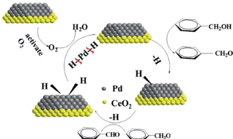
Fig. 44 Mechanism of the green oxidation method for benzyl alcohol with Pd/Fe<sub>3</sub>O<sub>4</sub>@mCeO<sub>2</sub> yolk-shell microspheres catalyst. This figure was adapted with permission from *Catalysis Letters*, 2016, 146, 1321–1330.<sup>283</sup>
