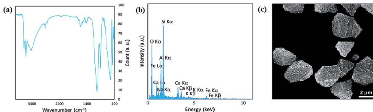
Fig. 41 (a) FT-IR spectrum, (b) EDX spectrum, and (c) SEM image of the recovered pumice microparticles after six recycling cycles. This figure was adapted with permission from *Research on Chemical Intermediates*, 2020, 46, 4113–4128.<sup>244</sup>
