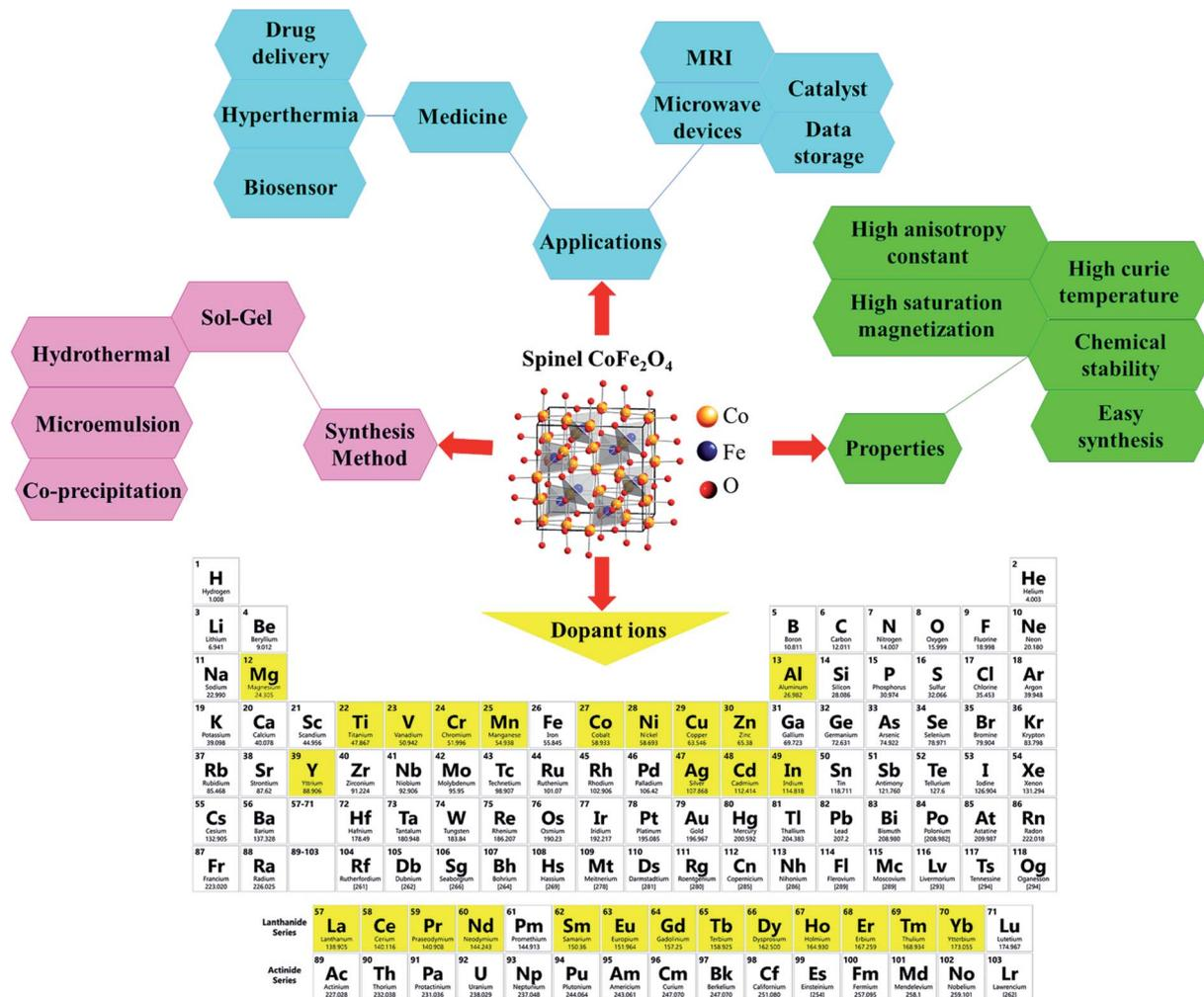
Fig. 6 Characteristics, synthesis methods, and applications of  $\text{CoFe}_2\text{O}_4$ . This figure was adapted with permission from *Ceramics International*, 2020, 46, 18391–18412.<sup>68</sup>
