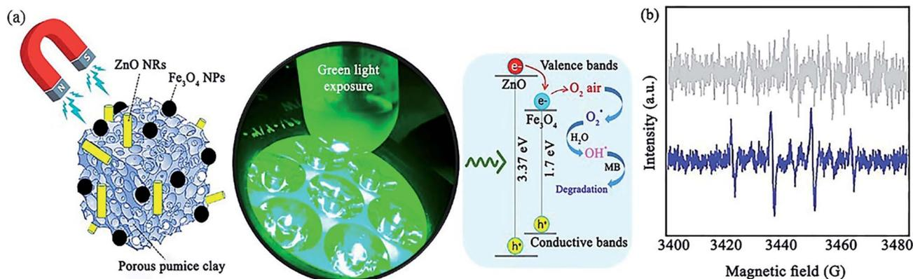
Fig. 24 (a) Illustration of the photocatalytic mechanism for the degradation of MB with synergistic effect between green light exposure and ZnO/Fe<sub>3</sub>O<sub>4</sub>@pumice photocatalyst. (b) ESR spectra for DMPO scavenger of ZnO/Fe<sub>3</sub>O<sub>4</sub>@pumice photocatalyst at ambient temperature. This figure was adapted with permission from *Materials Research Bulletin*, 2020, 130, 110946.<sup>148</sup>
