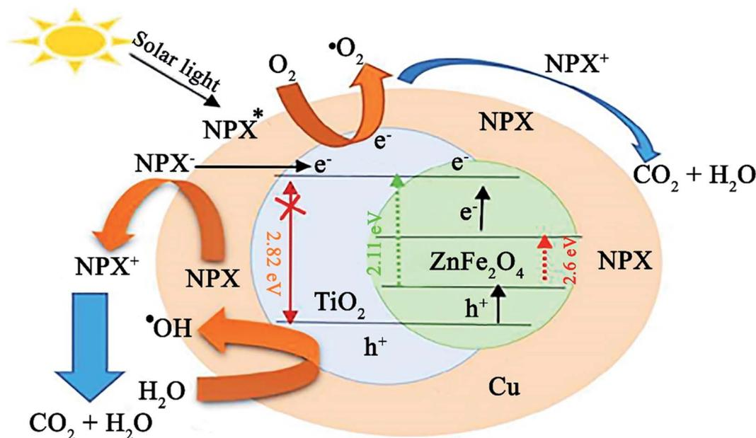
Fig. 23 Plausible mechanism for the photocatalytic degradation of NPX under a solar light source. This figure was adapted with permission from *Journal of Cleaner Production*, 2020, 268, 122023.<sup>146</sup>
