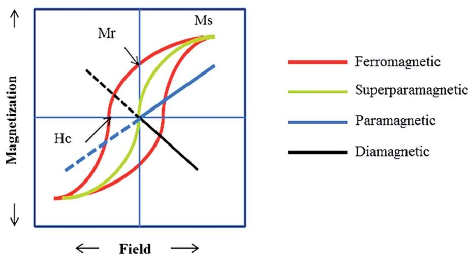
Fig. 36 Magnetic behavior under the influence of an applied field. This figure was adapted with permission from *Int. J. Mol. Sci.*, 2013, **14**, 15977–16009.<sup>230</sup>
