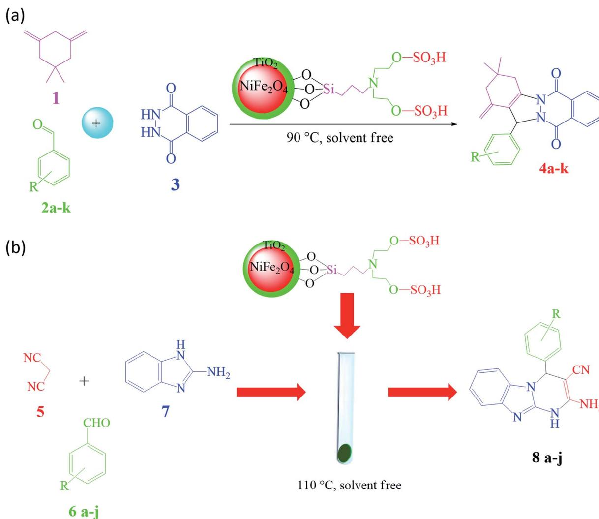
Fig. 32 (a) Schematic of the synthetic route for 2H-indazolo[2,1-b]phthalazine-triones. This figure was adapted with permission from *Chem. Sel.*, 2019, 4, 17–23.<sup>71</sup> (b) Schematic of the synthetic approach for benzo[4,5]imidazo[1,2-a]pyrimidines. This figure was adapted with permission from *Chem. Sel.*, 2019, 4, 17–23.<sup>71</sup>
