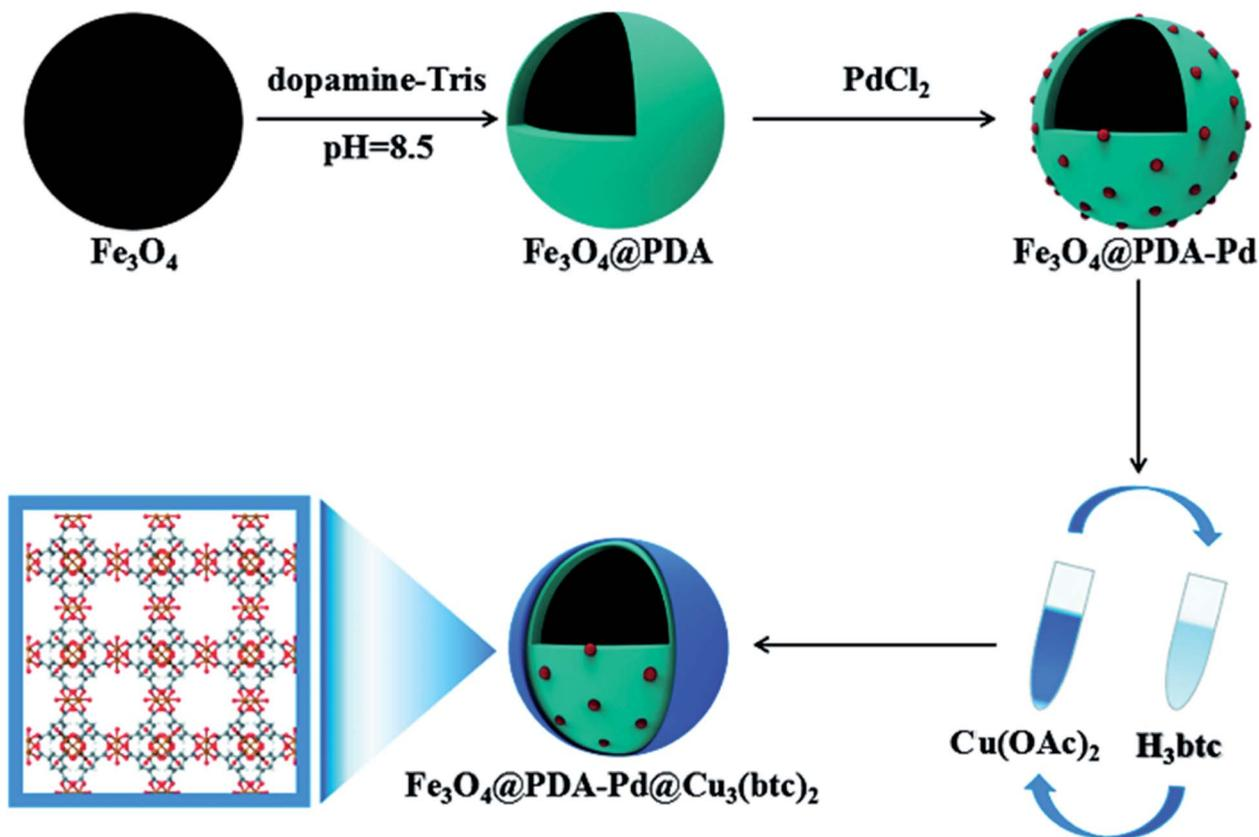
Fig. 9 Schematic of the procedure for the synthesis of the  $\text{Fe}_3\text{O}_4@\text{PDA-Pd}@\text{Cu}_3(\text{BTC})_2$  nanocomposite. This figure was adapted with permission from *ChemCatChem*, 2018, 10, 1446–1454.<sup>77</sup>
