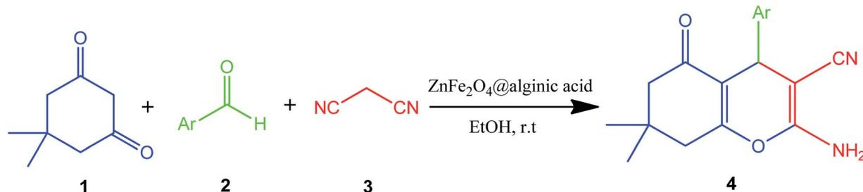
Fig. 34 Synthesis of 2-amino-3-cyano-4H-pyran derivatives at room temperature (r.t.). This figure was adapted with permission from: *Polyhedron*, 2019, 171, 193–202.<sup>75</sup>
