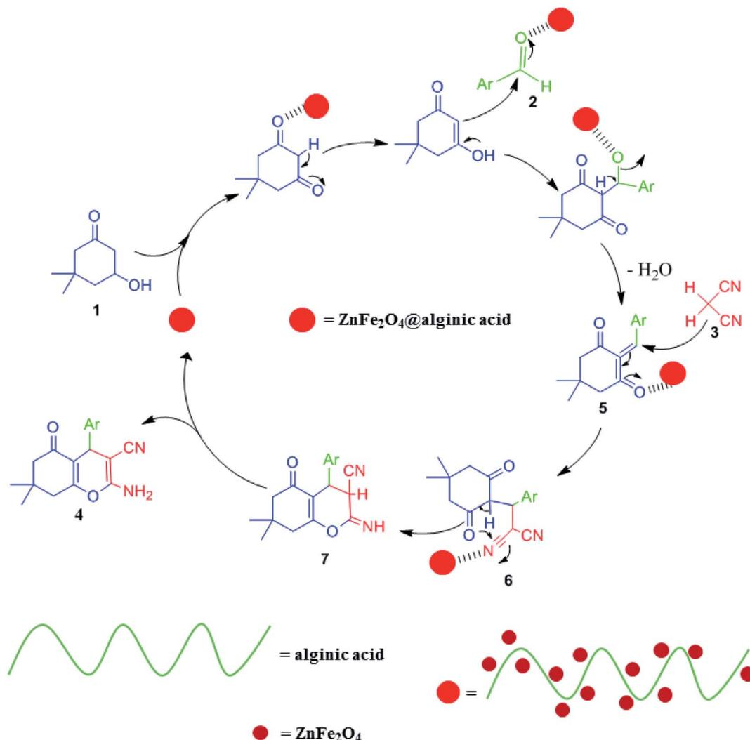
Fig. 35 Suggested mechanism for the synthesis of 2-amino-3-cyano-4H-pyran derivatives. This figure was adapted with permission from *Polyhedron*, 2019, 171, 193–202.<sup>75</sup>
