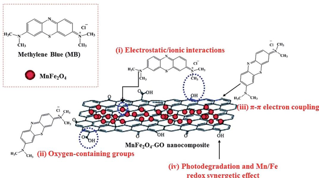
Fig. 25 Illustration of methylene blue (MB) adsorption mechanism on GO-MnFe<sub>2</sub>O<sub>4</sub> nanocomposites. This figure was adapted with permission from *RSC Advances*, 2018, 8, 12376–12389.<sup>154</sup>
