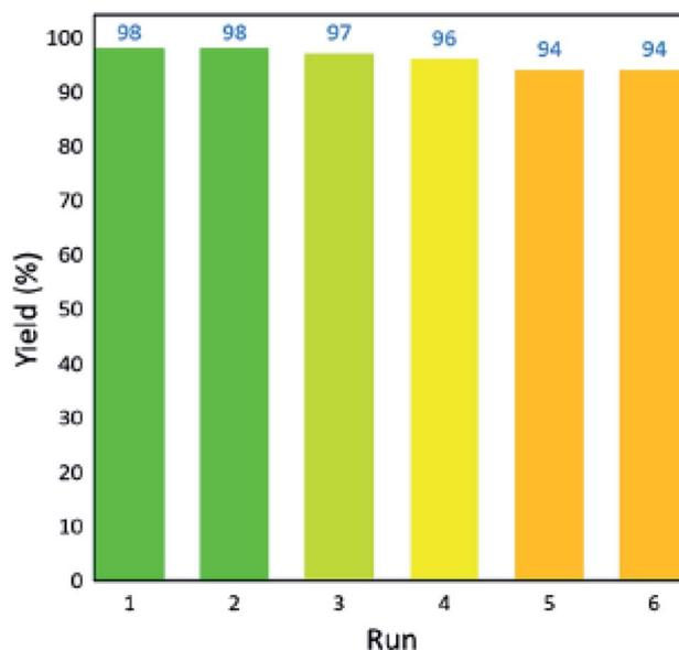
Fig. 40 Reusability diagram of the natural igneous pumice as a catalyst. This figure was adapted with permission from *Research on Chemical Intermediates*, 2020, 46, 4113–4128.<sup>244</sup>
