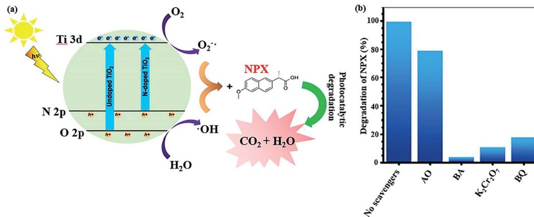
Fig. 22 (a) Mechanism for the photocatalytic decomposition of NPX by co-doped TiO<sub>2</sub>. (b) NPX degradation efficiency with the photocatalyst in the presence and absence of various scavengers. This figure was adapted with permission from *Journal of Environmental Science and Health, Part A*, 2019, 54, 1254–1267.<sup>145</sup>
