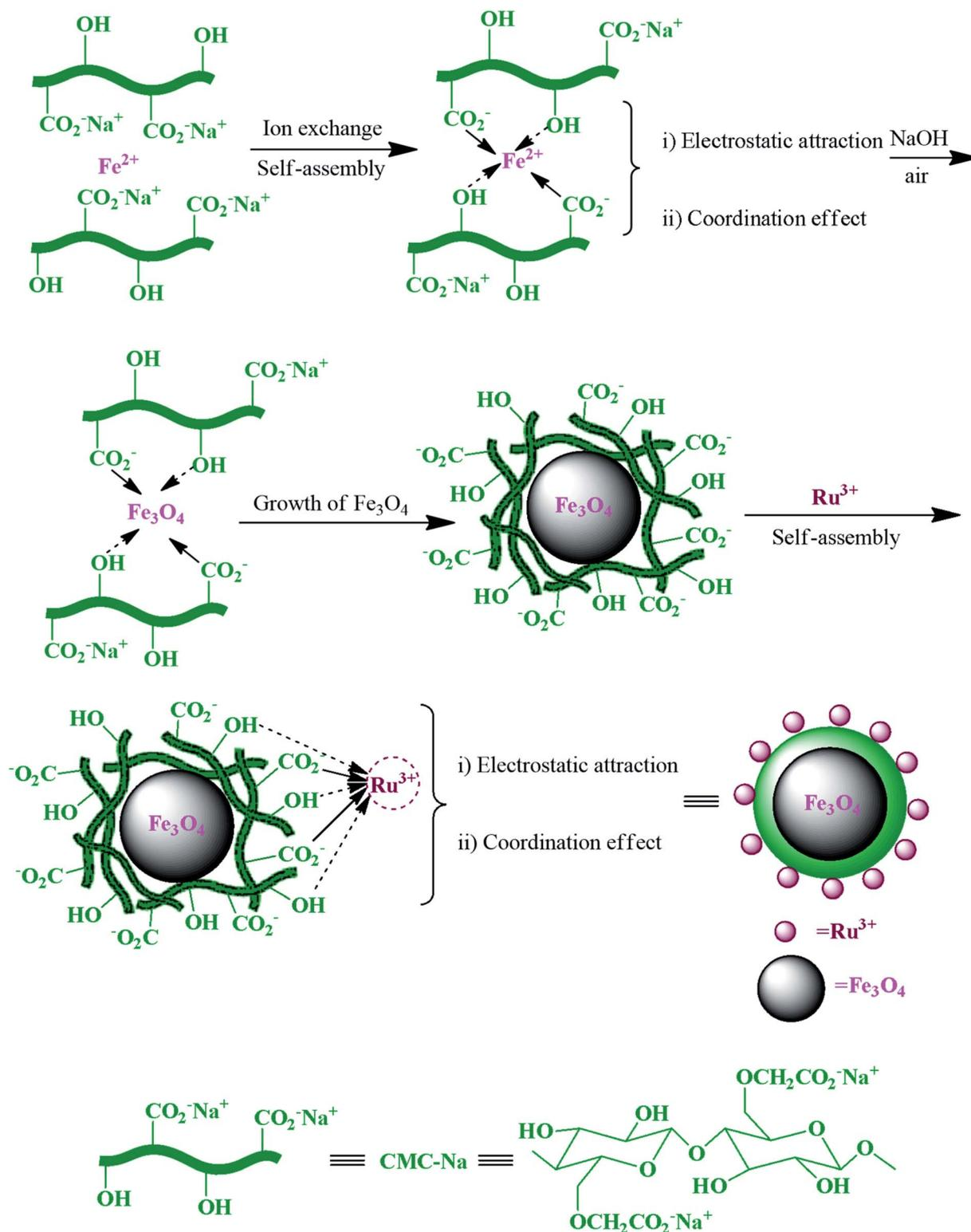
Fig. 16 Schematic of the preparation of magnetic  $\text{Ru}^{\text{III}}@ \text{CMC}/\text{Fe}_3\text{O}_4$  organic/inorganic hybrid catalyst via self-assembly. This figure was adapted with permission from: *Molecular Diversity*, 2019, 23, 421–442.<sup>103</sup>
