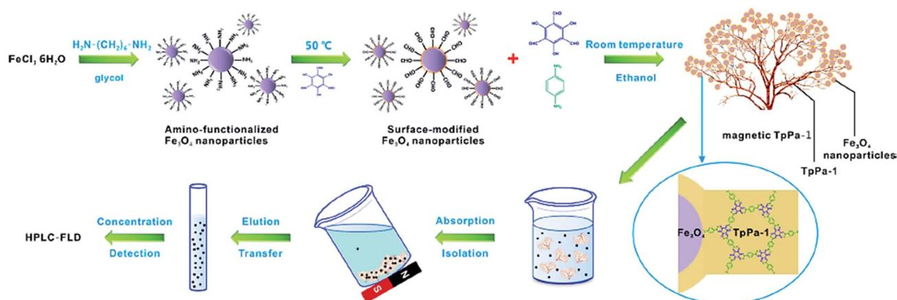
Fig. 11 Schematic showing the synthesis and function of the bouquet-like magnetic TpPa-1 sorbent. This figure adapted with permission from ACS Applied Materials & Interfaces, 2017, 9, 2959–2965.<sup>87</sup>
