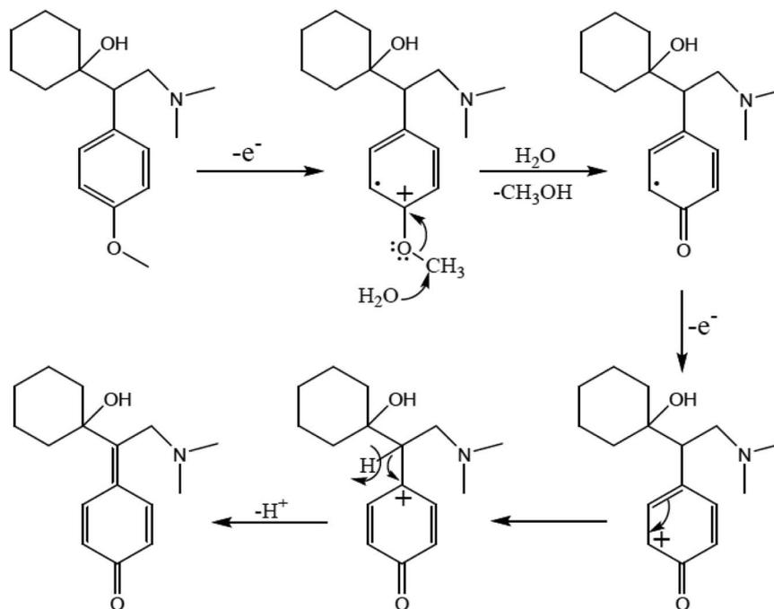
Fig. 28 Proposed mechanism for the electrooxidation of venlafaxine at the surface of  $\text{Fe}_3\text{O}_4$ @nano-cellulose/Cu nanocomposite/GSPE. This figure was adapted with permission from *Industrial & Engineering Chemistry Research*, 2020, 59, 4219–4228.<sup>41</sup>
