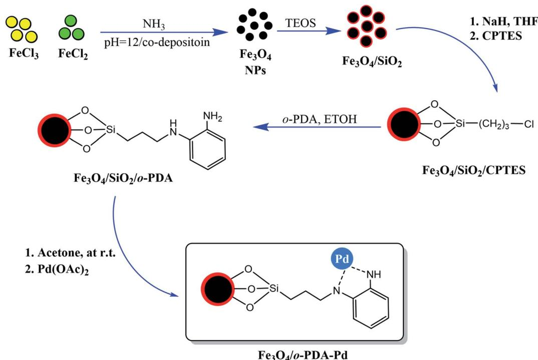
Fig. 5 Preparation of Fe<sub>3</sub>O<sub>4</sub>/o-PDA-Pd heterogeneous magnetic nanocatalyst. This figure was adapted with permission from *Journal of Physics and Chemistry of Solids*, 2020, **136**, 109200.<sup>17</sup>
