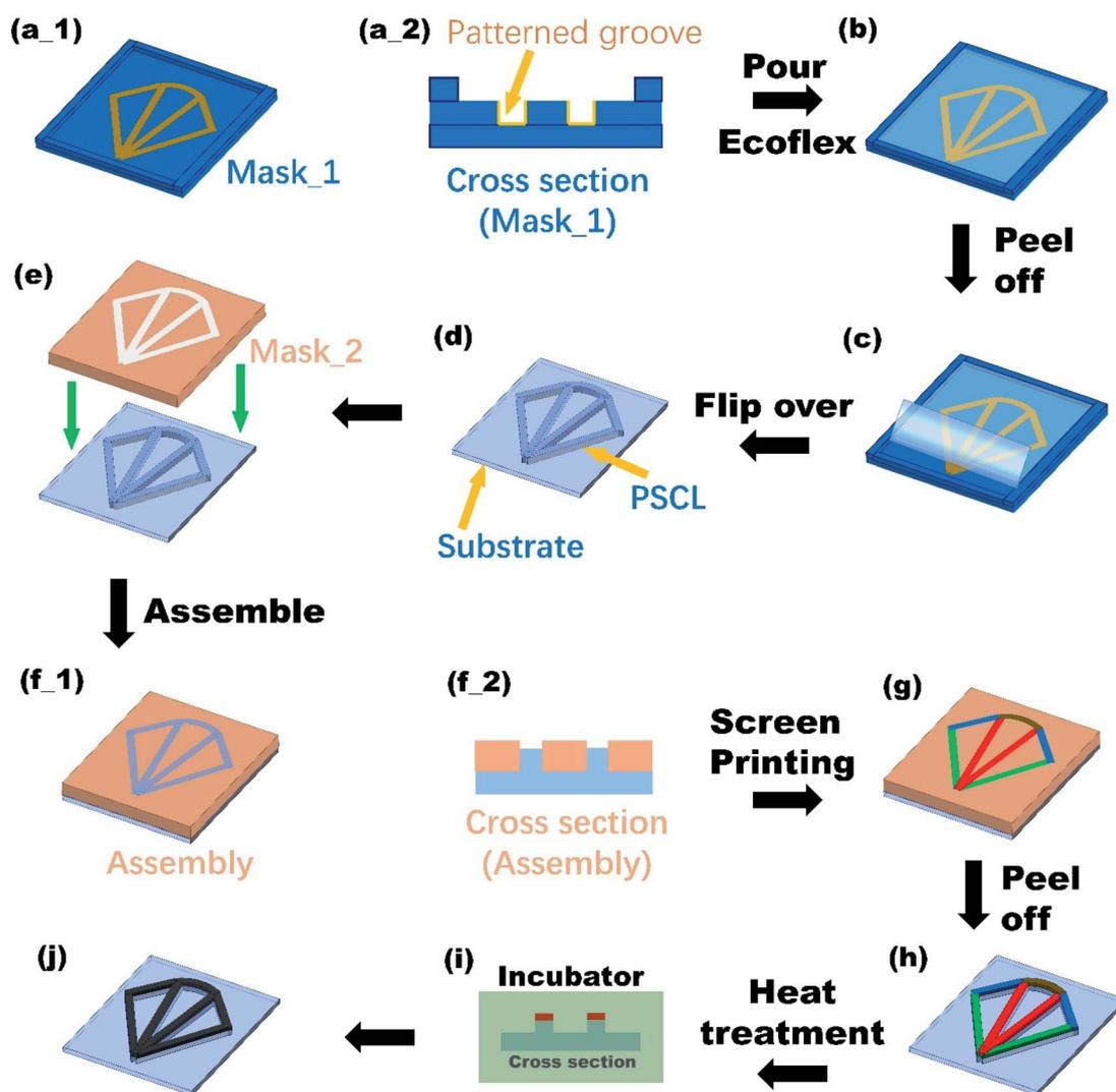
Fig. 2 Fabrication process of the samples. (a<sub>1</sub>) and (a<sub>2</sub>) The intaglio mold and the cross-section. (b) Eco-flex pouring. (c) Substrate peeling off. (d) Substrate flipping over. (e) Mask 2 and substrate assembling. (f<sub>1</sub>) and (f<sub>2</sub>) The assembly and the cross section. (g) Screen printing. (h) Sensor peeling off. (i) Heat treatment. (j) 3D schematic of the sensor.
