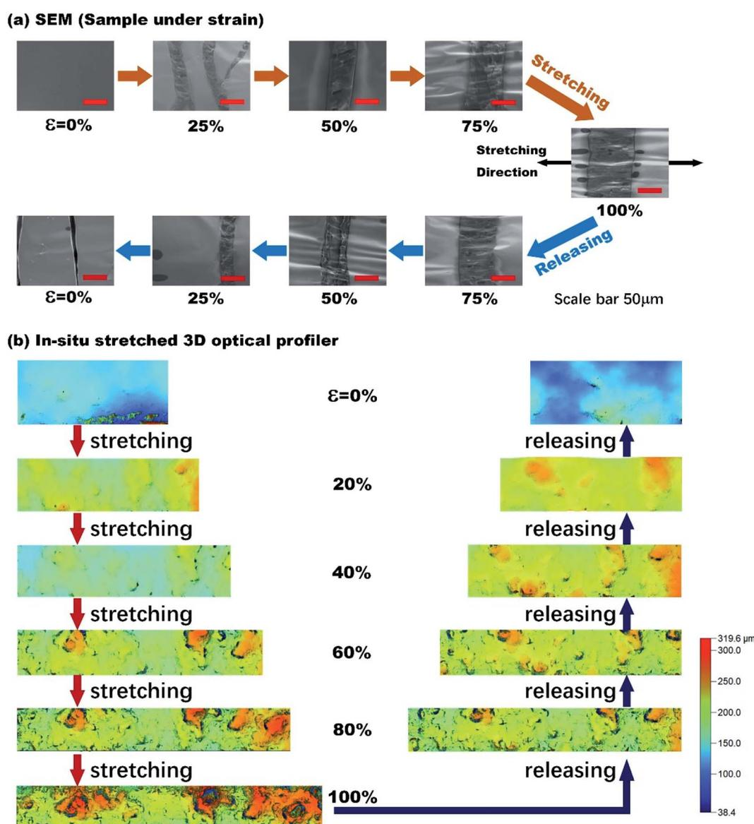
Fig. 5 Crack evolution of nanocomposites during stretching. (a) SEM images of the microcracks in nanocomposites under tensile strains. (b) 3D surface topography of the nanocomposites during *in situ* stretching.
