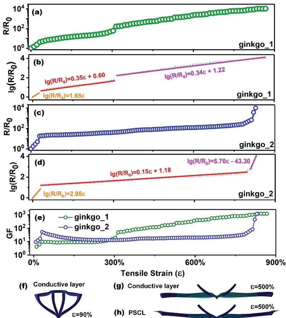
Fig. 3 Electrical and stretchable properties. (a) Resistance change rate of the sensor with the ginkgo\_1 pattern. (b) The logarithmic linear fit. (c) Resistance change rate of the sensor with the ginkgo\_2 pattern. (d) The logarithmic linear fit. (e) Gauge factor of these two sensors. ANSYS simulation of the pattern deformation during stretching for (f) conductive layer at 90% strain, (g) conductive layer at 500% strain and (h) PSCL at 500% strain.
