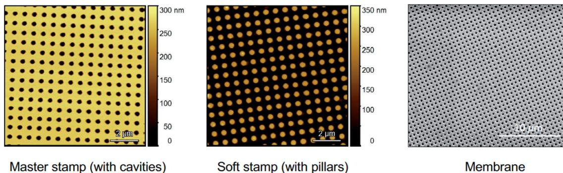
Fig. 2 (a and b) AFM images of the (a) master stamp and (b) soft stamp; (c) SEM images of the membrane fabricated *via* NIL.
