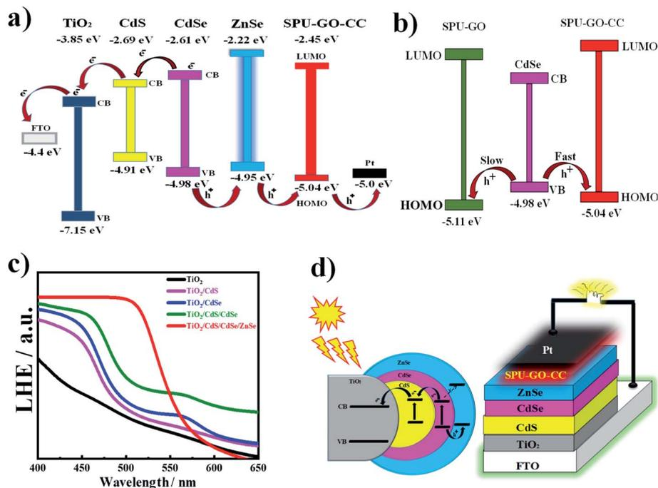
Fig. 5 (a) Energy profile diagram of TiO<sub>2</sub>, CdS and CdSe with SPU-GO-CC gel electrolyte; (b) comparison of the energy level of the SPU-GO and SPU-GO-CC with CdSe QDs showing the transport behaviour of holes; (c) light-harvesting efficiency of layer by layer deposition of QDs photoanodes FTO/TiO<sub>2</sub>, FTO/TiO<sub>2</sub>/CdS, FTO/TiO<sub>2</sub>/CdS/CdSe and ZnSe passivation layer; and (d) solar excitation mechanism and layered structure of fabricated QDSSCs.
