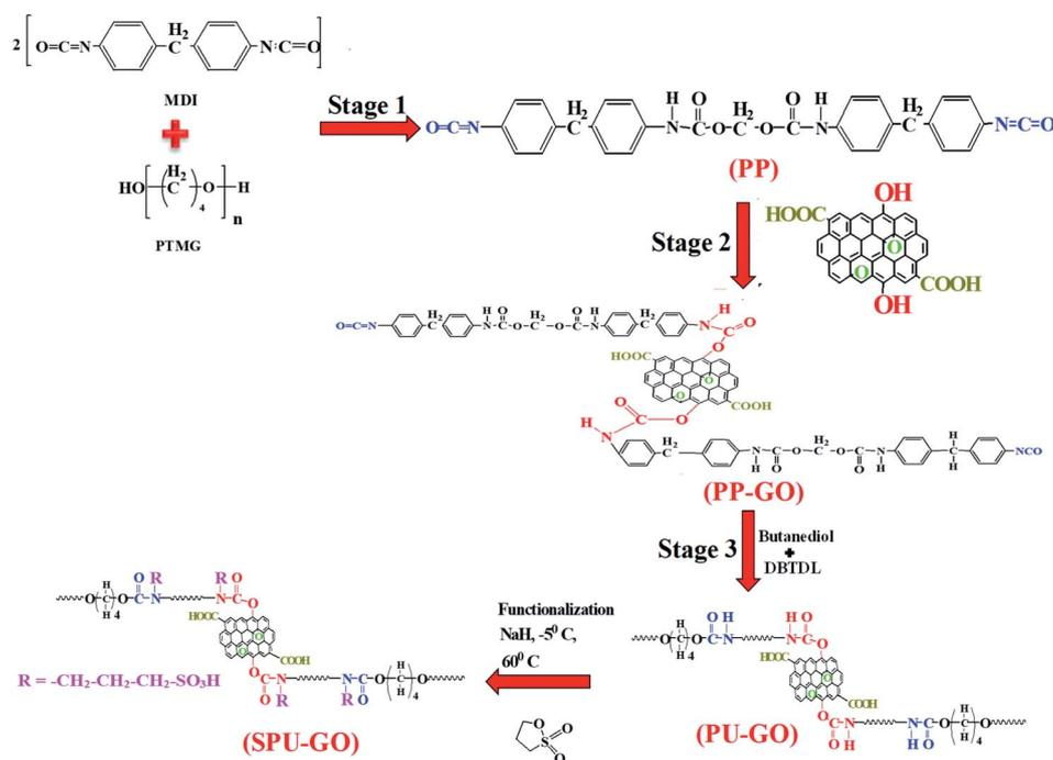
**Scheme 1** A reaction scheme for the synthesis of GO-tagged polyurethane (PU-GO) in three stages and its subsequent functionalization (SPU-GO). The designation of polymer is mentioned below with the respective chemical formula.
