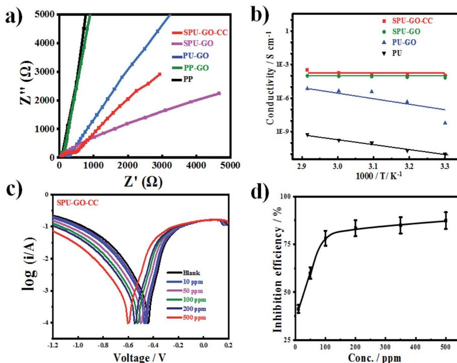
Fig. 2 (a) Nyquist plots for the indicated pure and functionalized PUs; (b) Arrhenius plots of the pure and indicated functionalized polymers; (c) potentiodynamic polarization measurement of mild steel with and without the indicated inhibitors in 0.5 M H<sub>2</sub>SO<sub>4</sub> solution; and (d) percentage inhibition efficiency as a function of inhibitor (SPU-GO-CC) concentration.
