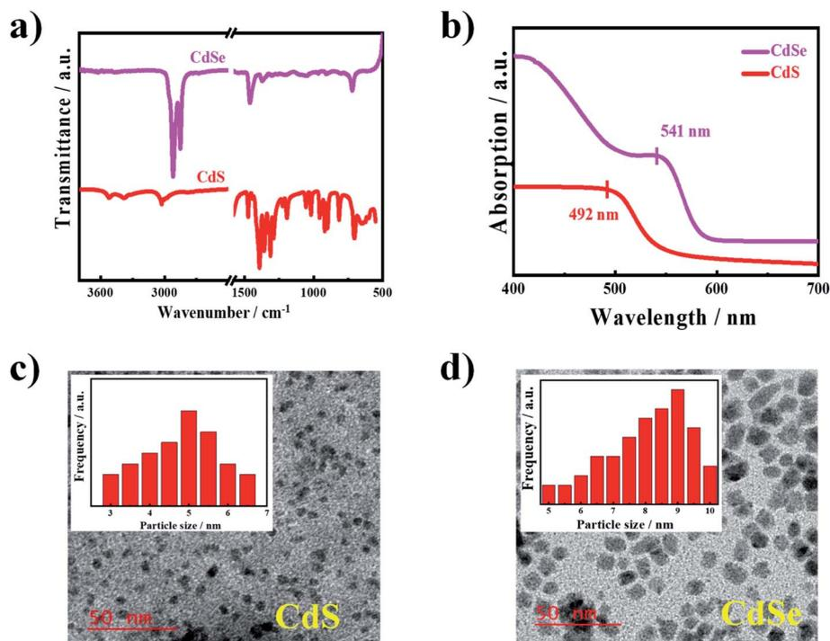
**Fig. 3** (a) UV-vis absorption spectra of CdS and CdSe showing the absorption peak; (b) FTIR spectra of the synthesised CdS and CdSe QDs; (c) TEM bright-field image and particle distribution of CdS QDs; and (d) TEM bright-field image and particle size distribution of CdSe QDs.
