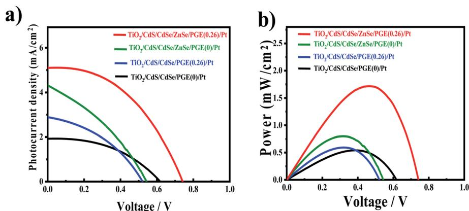
Fig. 6 (a)  $J$ - $V$  characteristics measurement to calculate the photocurrent density and open-circuit voltage under 1 Sun illumination ( $100 \text{ mW cm}^{-2}$ ); and (b) power-voltage curve to calculate the power conversion efficiency (PCE) of the indicated QDSSCs.
