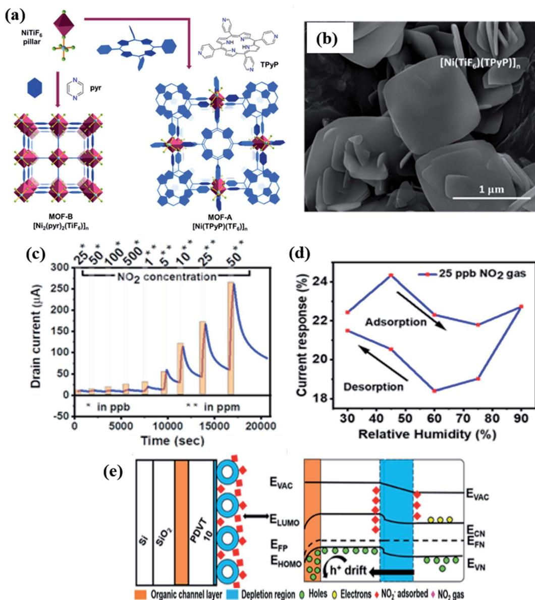
Fig. 22 (a) Schematic diagram of the preparation of the  $[\text{Ni}(\text{TPyP})(\text{TiF}_6)]_n$  MOF, (b) SEM images of MOF-A  $[\text{Ni}(\text{TPyP})(\text{TiF}_6)]_n$ , (c) sensing properties towards  $\text{NO}_2$  gas, (d) humidity effect of the OFET gas sensor, and (e) sensing mechanism of PVDT-10 and MOF based OFET sensors.<sup>177</sup>
