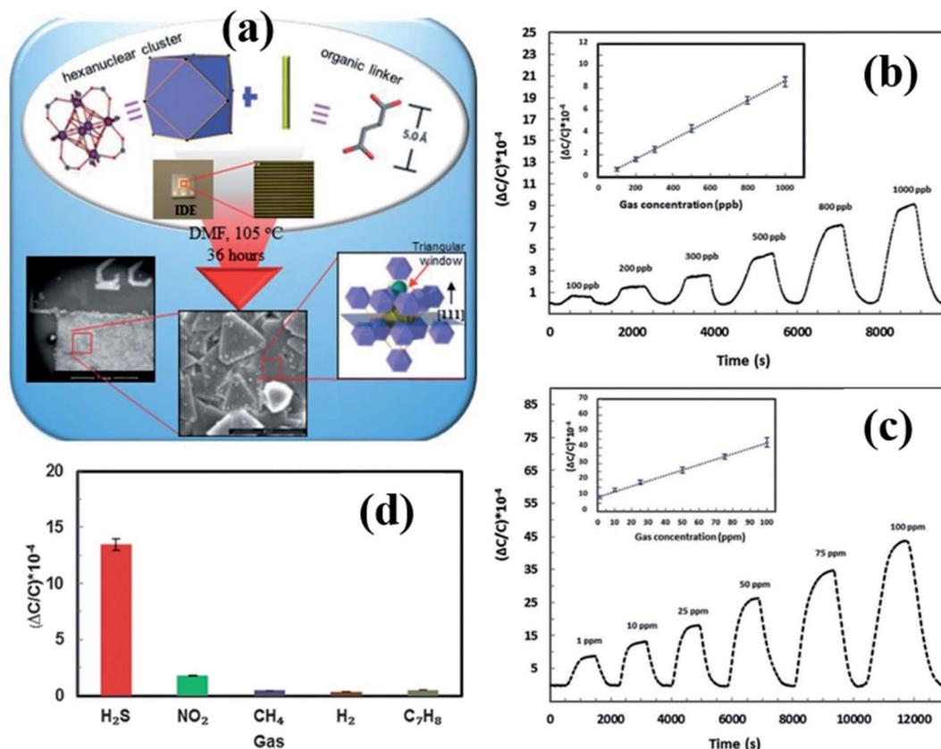
Fig. 16 (a) The schematic diagram of the preparation of the fum-fcu-MOF by the solvothermal method and its integration onto the IDE, (b and c) capacitive response transients of the fum-fcu-MOF sensor for the ppb and ppm levels of H<sub>2</sub>S detection, and (d) the selectivity test of the fum-fcu-MOF sensor towards different interfering gases. Reprinted from ref. 137, copyright@2021, Wiley and Sons.
