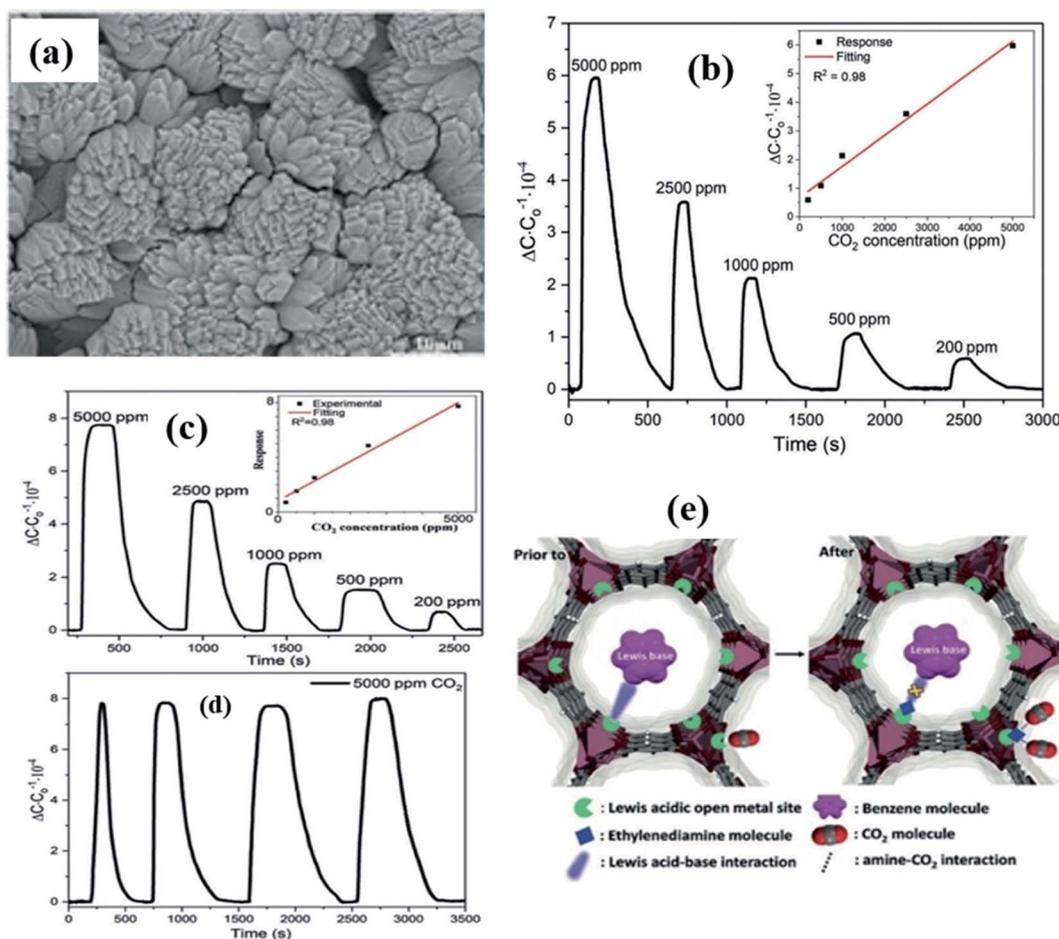
Fig. 19 (a) SEM image of the as grown Mg-MOF-74 on the IDE substrate, (b and c) capacitive response transients towards CO<sub>2</sub> at RT and after ethylenediamine-functionalization, (d) repeatability study of the ethylenediamine-functionalized Mg-MOF-74 sensor for 5000 ppm and (e) schematic diagram of the sensing mechanism of Mg-MOF-74. Reprinted from ref. 139, copyright@2021, John Wiley and Sons.
