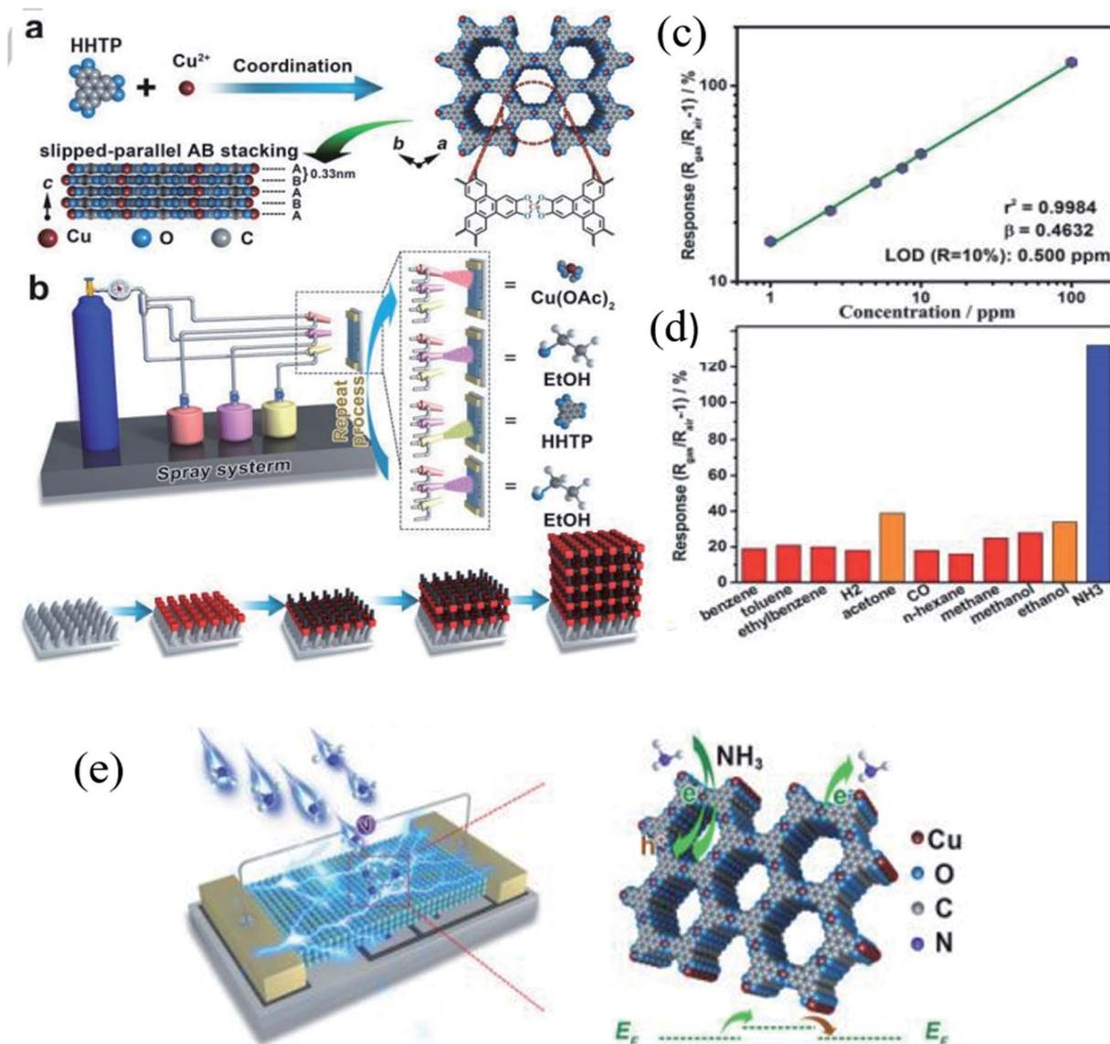
Fig. 3 (a) Illustration of the crystal structure of  $\text{Cu}_3(\text{HHTP})_2$ . (b) Fabrication of the  $\text{Cu}_3(\text{HHTP})_2$  thin film by a spray layer-by-layer (LBL) method using the LPE technique, (c) LOD graph, (d) selectivity test of the  $\text{Cu}_3(\text{HHTP})_2$  thin-film sensor, and (e)  $\text{NH}_3$  sensing mechanism of the  $\text{Cu}_3(\text{HHTP})_2$  thin film sensor at RT. Reproduced from ref. 70 with permission from Wiley Sons, copyright 2021.
