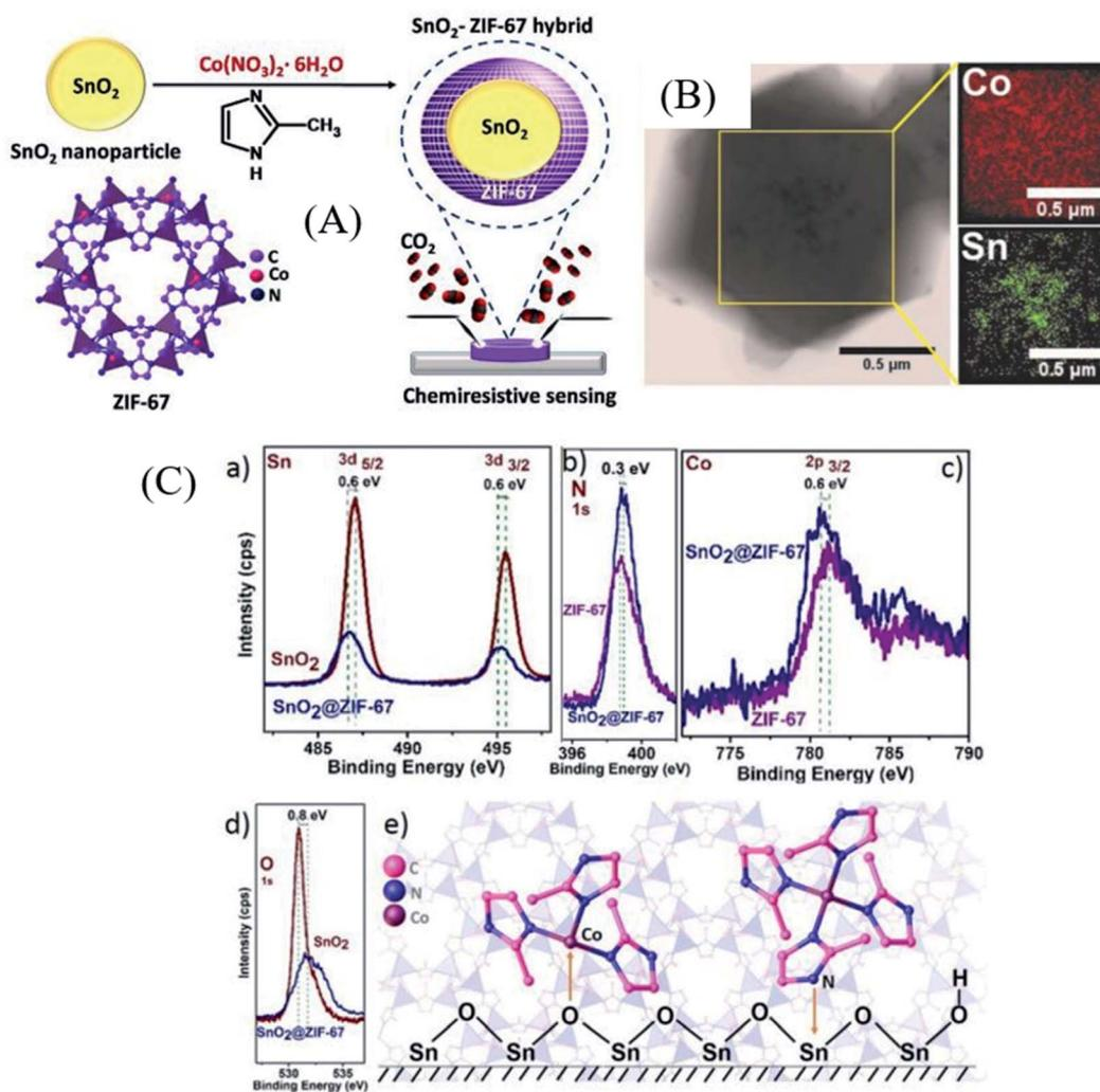
Fig. 9 (A) Schematic illustration of  $\text{SnO}_2$ @ZIF-67 architecture formation, (B) TEM image of the core-shell  $\text{SnO}_2$ @ZIF-67 material with its corresponding EDX-elemental analysis, and (C) XPS analysis to examine the synergistic effect of  $\text{SnO}_2$  and the ZIF-67 MOF. Reproduced from ref. 101 with permission from Wiley-VCH GmbH, copyright 2021.
