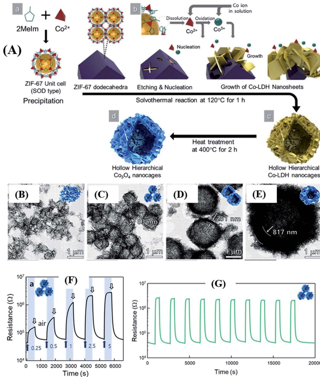
Fig. 6 (A) Synthesis protocol of hierarchical hollow  $\text{Co}_3\text{O}_4$  nanocages using ZIF-67 as the template, (B–E) SEM images of  $\text{Co}_3\text{O}_4$  hierarchical hollow nanocages (HHN) with different sizes, (F) response/recovery curves of the 10- $\text{Co}_3\text{O}_4$  sensor tested at 225 °C towards *p*-xylene (0.5–2.5 ppm), and (G) repeatability test at 225 °C. Reprinted from ref. 88 with permission from American Chemical Society, copyright 2021.
