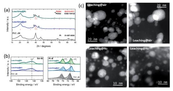
Fig. 1 (a) Powder XRD patterns (b) Gd 4d and Pt 4f photoemission lines; and (c) high-angle annular dark field STEM micrographs of the Pt<sub>x</sub>Gd/C catalysts washed under air- or N2-atmosphere. 40% Pt/C from Johnson-Matthey is used as reference in (a) and (b).
