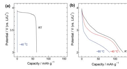
Fig. 8 The discharge curves for (a)  $LiCoO_2$  and (b) SWCNT@PB
