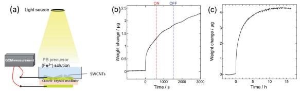
Fig. 5 (a) QCM experiment (b) in situ tracking of electrode mass during synthesis and (c) extended time tracking of the synthesis process
