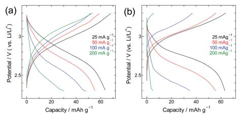
Fig. 10 Charge/discharge curves for the SWCNT@PB composite at (a) room temperature and (b)  $-40\,^{\circ}$ C.
