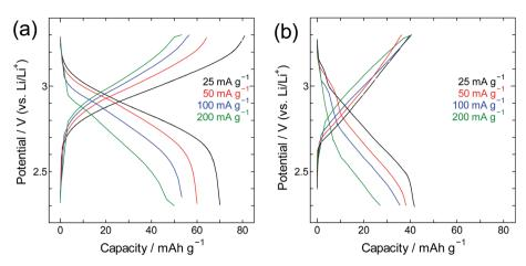
Fig. 9 Charge/discharge curves for PB crystals at (a) room temperature and (b) -40 °C.
