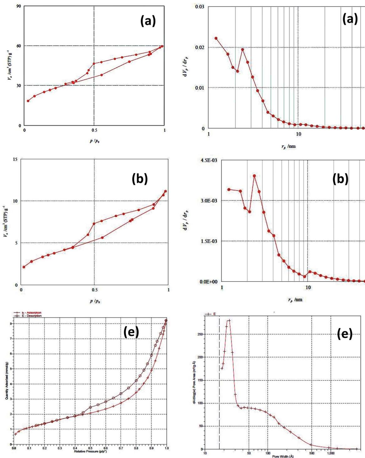
Fig. 4 N<sub>2</sub> adsorption–desorption isotherms of PMAMOSa,b,e (1) obtained using the PMDADA precursor I prepared in THF (a) or DMF solvent (b) with the simultaneous addition of precursor I and TEOS to the mixture of HCl and Pluronic P123. CTAB was dissolved in ammonia solution and used as the template (e).
