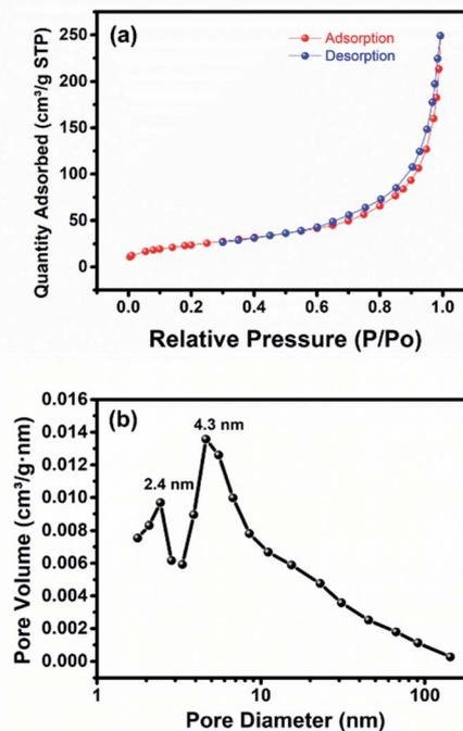
Fig. 3 (a) N<sub>2</sub> adsorption/desorption isotherm and (b) practical size distribution of the as-prepared Ti–Mo–Ni nanoparticles *via* breakdown anodization.
