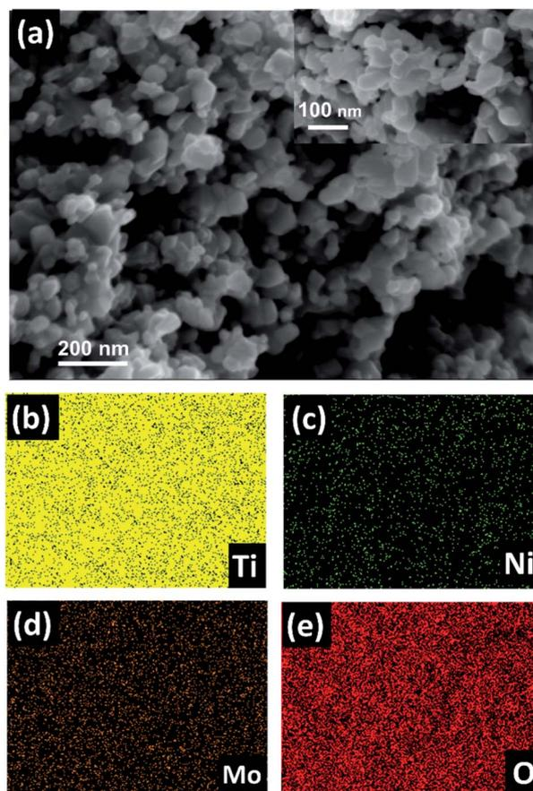
Fig. 1 (a) FESEM image and (b–e) EDX elemental mapping of the as-prepared nanoparticles *via* breakdown anodization of the Ti–Mo–Ni sheet in a 0.1 M HClO<sub>4</sub> aqueous electrolyte at 20 V.
