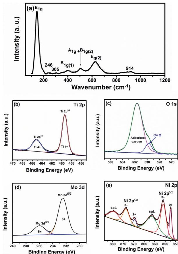
Fig. 2 (a) Raman and (b–e) high resolution XPS spectra: (b) Ti 2p, (c) O 1s, (d) Mo 3d, and (e) Ni 2p of the as-prepared nanoparticles via breakdown anodization of the Ti–Mo–Ni sheet in a 0.1 M HClO<sub>4</sub> aqueous electrolyte at 20 V.
