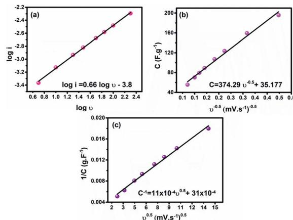
Fig. 5 (a) Current-scan rate relationship, (b) dependence of  $C$  on  $v^{-0.5}$ , and (c) dependence of  $1/C$  on  $v^{0.5}$  for the as-prepared electrode.
