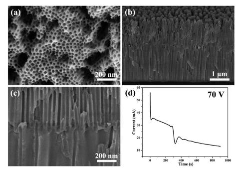
Fig. 2 (a-c) The SEM images of anodic ZrO<sub>2</sub> nanotubes anodized at a constant voltage of 70 V for 900 s. (d) The corresponding current-time curve over 900 s.
