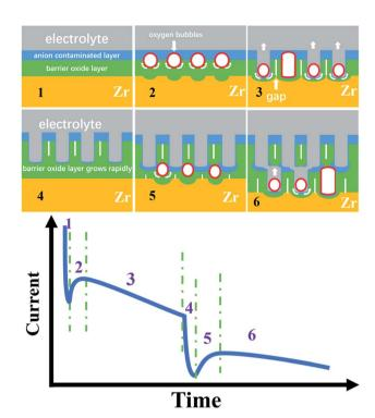
Fig. 4 Schematic diagram of the three stages and six stages of growth of anodic ZrO<sub>2</sub> nanotubes.
