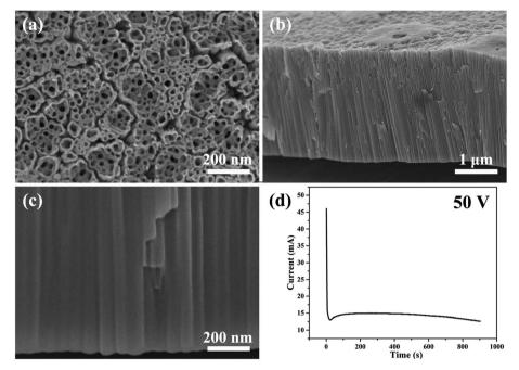
Fig. 1 (a-c) The SEM images of anodic ZrO<sub>2</sub> nanotubes anodized at a constant voltage of 50 V for 900 s. (d) The corresponding current-time curve over 900 s.
