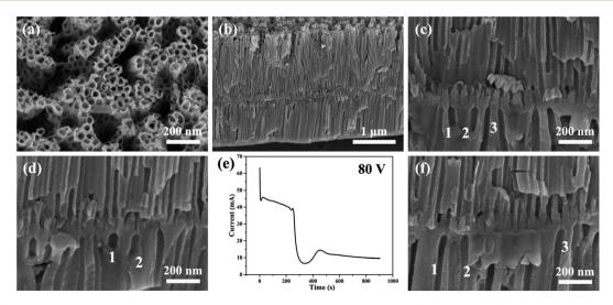
Fig. 3 (a-d, f) The SEM images of anodic ZrO<sub>2</sub> nanotubes anodized at a constant voltage of 80 V for 900 s. (e) The corresponding current-time curve over 900 s.
