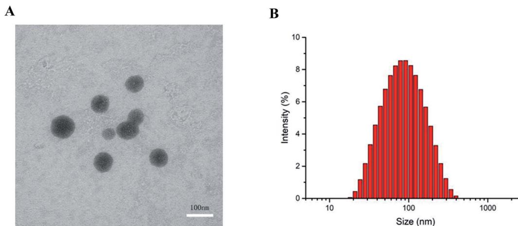
Fig. 4 (A) TEM image of S4A-BSA-Au NPs (bar = 100 nm). (B) Size distribution of S4A-BSA-Au NPs measured by the DLS technique.
