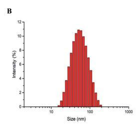
Fig. 2 (A) TEM image of B-BANC-NPs (bar = 100 nm). (B) Size distribution of B-BANC-NPs measured by the DLS technique.
