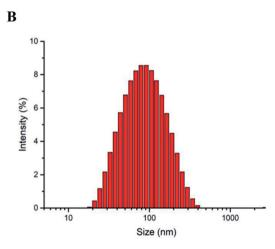
(A) TEM image of S4A-BSA-Au NPs (bar = 100 nm). (B) Size distribution of S4A-BSA-Au NPs measured by the DLS technique.
