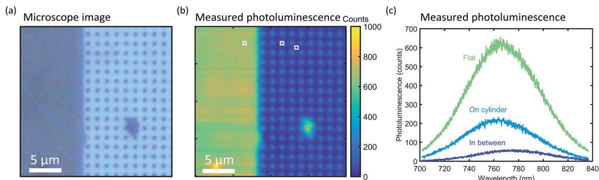
**Fig. 3** Photoluminescence mapping after thick QD print. (a) Microscope image of the Si substrate (blue) with a thick QD layer on top of flat Si and the Si cylinder array (gray). (b) PL map of the area depicted in (a). Color scale depicts the intensity at 760 nm wavelength. (c) PL spectra of three typical positions on the sample, indicated by the squares in (b): on the flat Si (green), in the middle of a cylinder (light blue), and in between four cylinders (dark blue).
