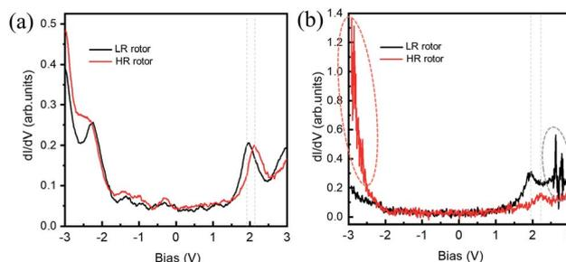
Fig. 3 (a)  $dI/dV$  spectra obtained on the LR (black curve) and HR (red curve) rotors with a large tip-sample distance. (b)  $dI/dV$  spectra obtained on the LR (black curve) and HR (red curve) rotors with a small tip-sample distance. The regions of current fluctuation are highlighted by dotted ovals. Initial condition:  $V_b = -3.0$  V and  $I_t = 50$  pA for (a);  $V_b = -3.0$  V and  $I_t = 400$  pA for (b).
