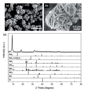
Fig. 2 SEM images (a and b) and XRD pattern (c) of the desert-rose-like WS $_3$  synthesized by the sulphurization of the WO $_3$ ·0.33H $_2$ O microspheres. XRD patterns of the possible W compounds and W element are shown in panel (c).
