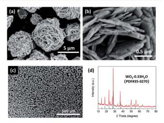
Fig. 1 Scanning electron microscopy (SEM) images (a–c) and XRD pattern (d) of the desert-rose-like  $WO_3 \cdot 0.33H_2O$  microspheres, which were used as the starting materials to synthesize  $WS_3$ .
