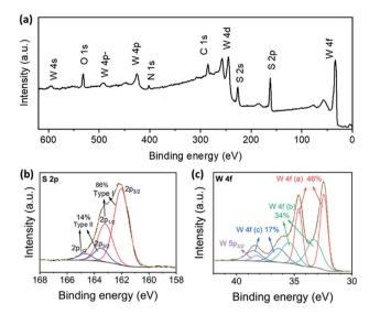
Fig. 3 XPS spectra of WS $_3$ . The predominant elements in the substance were W and S, as shown in the survey spectrum (a). Two types of S were found from the peak fitting result of the S 2p region (b), indicating the existence of bridging S $_2$ <sup>2</sup> or apical S<sup>2</sup>. Three types of W 4f were found from the peak fitting result of the W 4f region (c), which indicated a mixed valence state of +4 and higher ones and complex chemical environments of W.
