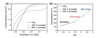
Fig. 6 Activity of WS<sub>3</sub> as the electrochemical catalyst for the HER. Polarization curves (a) and Tafel curves (b) of as-prepared WS<sub>3</sub>, and WS<sub>3</sub> annealed at 300 °C and 600 °C are shown respectively.
