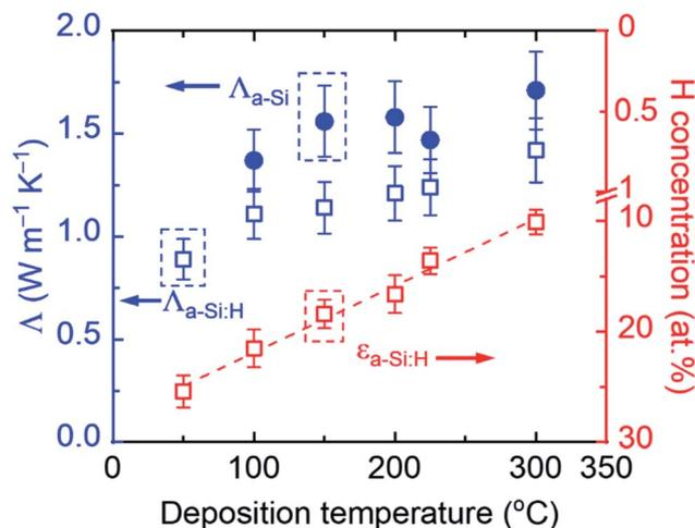
Fig. 3 The room-temperature thermal conductivity (left axis) and H concentration (right axis) of PECVD a-Si:H films as a function of the deposition temperature.  $\epsilon_{\text{a-Si:H}}$  represents the H concentration of the as-produced samples. The dashed line shows the linear dependence of H concentration on deposition temperature.  $\Lambda_{\text{a-Si:H}}$  and  $\Lambda_{\text{a-Si}}$  are the room-temperature thermal conductivities of the as-produced and annealed films, respectively.
