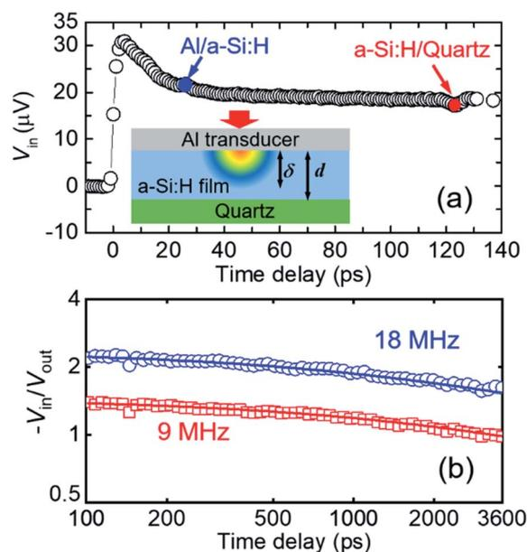
**Fig. 2** (a) Picosecond acoustics measurements of an a-Si:H film deposited on quartz. The inset is the sample stack for thermal conductivity measurements. (b) Representative TDTR signals of the a-Si:H film (10.1 at%) with two modulation frequencies. The solid lines are the fitting curves following a heat diffusion model, which give a thermal conductivity of 1.42 W m<sup>-1</sup> K<sup>-1</sup>.
