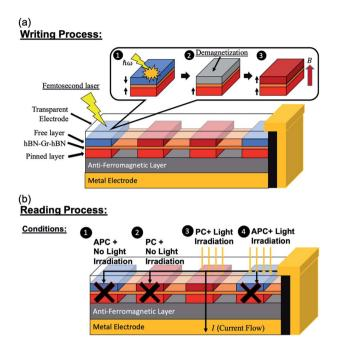
Fig. 7 (a) The writing and (b) the reading process of the proposed Ni/ hBN-Gr-hBN/Ni MTJ device with light irradiation
