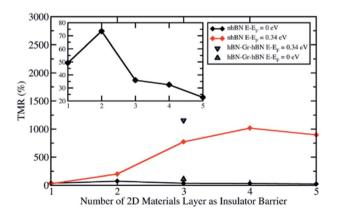
Fig. 2 The TMR ratio vs. the number of 2D material layers as a tunnel barrier at two different energies;  $E-E_{\rm F}=0$  eV (the zero-bias limit) and 0.34 eV (the highest peak of spin-down electron transmission probability in the PC state started from n=3).
