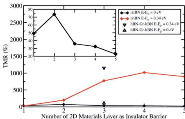
Fig. 2 The TMR ratio vs. the number of 2D material layers as a tunnel barrier at two different energies;  $E - E_F = 0$  eV (the zero-bias limit) and 0.34 eV (the highest peak of spin-down electron transmission probability in the PC state started from  $n = 3$ ).
