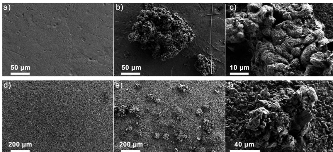
Fig. 6 SEM micrographs: (a) fresh Na, (b) Na electrode after stripping and deposition; (c) higher magnification of Na deposits, (d) fresh CC@1400 °C electrode, (e) CC@1400 °C electrode after the plating test, and (f) higher magnification of the plated CC@1400 °C electrode.
