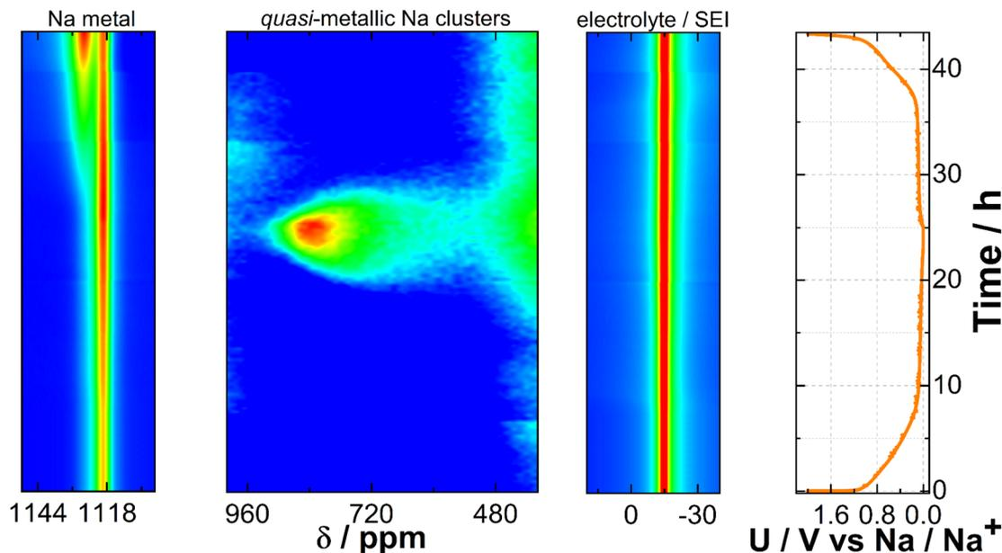
Fig. 3  $^{23}\text{Na}$  *operando* solid-state NMR spectrum for the Na||CC@1400 °C half cell at 90° orientation with respect to the external magnetic field of the spectrometer. First cycle electrochemistry is shown on the right.
