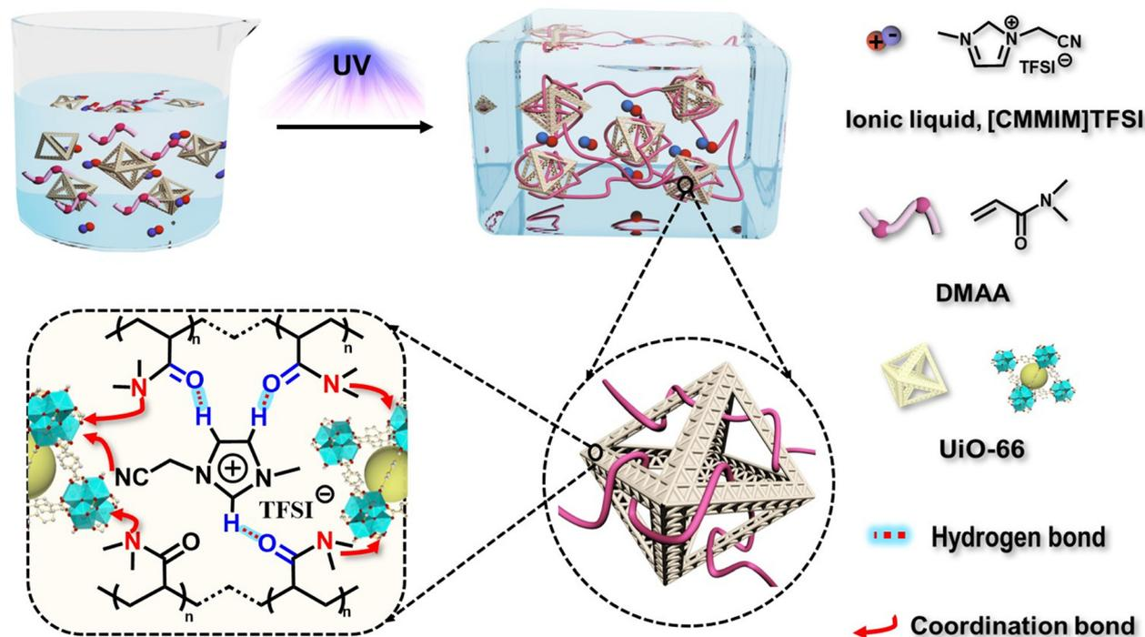
**Scheme 1** Schematic of the preparation of UiO-66-ionogels. UiO-66 was mixed with *N,N*-dimethylacrylamide (DMAA), and 1-cyanomethyl-3-methylimidazolium bis[(trifluoromethyl)sulfonyl]imide ([CMMIM][TFSI]), which resulted in the formation of a linear network with interpenetrating entangled topology after polymerization of the monomers. The polymer chains and [CMMIM][TFSI] interacted with the metal sites of UiO-66 and thus formed physically crosslinked UiO-66-ionogels.
