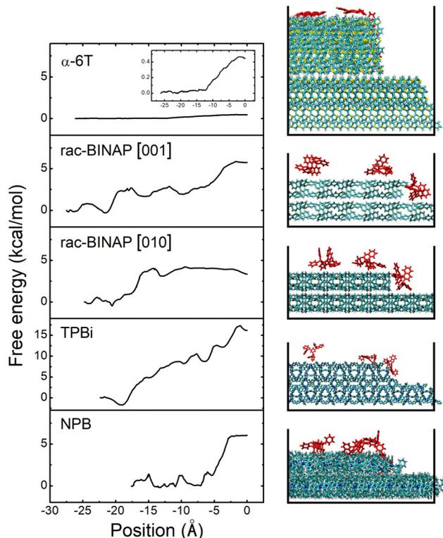
Fig. 4 Trajectories of  $\alpha$ -6T, *rac*-BINAP, TPBi and NPB molecules during a step-edge descent and their respective free energy profiles. The molecule's position at the step-edge after descent corresponds to 0 Å. For *rac*-BINAP the trajectories in both the [010] and [001] directions are shown.
