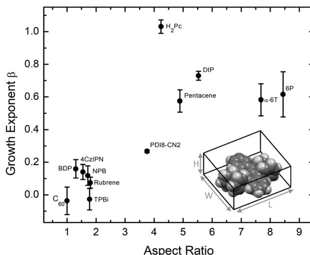
Fig. 3 Growth exponent  $\beta$  versus molecular aspect ratio. The aspect ratio is defined as the longest dimension divided by the shortest dimension of a box containing a given molecule, as illustrated in the lower-right for rubrene. Errors bars show one standard deviation of the fit data.
