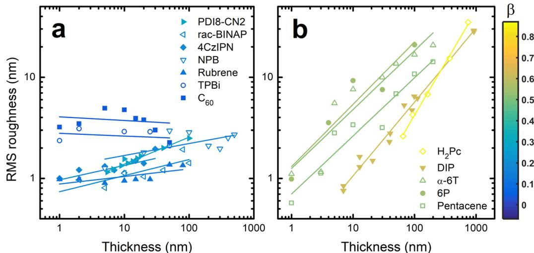
Fig. 2 Root mean square roughness versus film thickness for materials considered in this work and from literature. The data are separated for clarity with the materials that remain smooth (lower  $\beta$ ) in (a) and materials that become rough (higher  $\beta$ ) in (b). The color of each data set corresponds the slope of the fit line, which is equal to the growth exponent,  $\beta$ .
