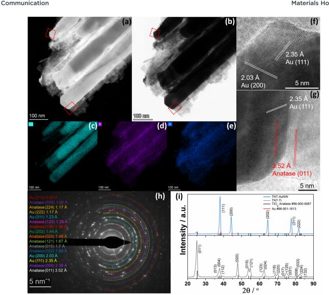
Fig. 3 (a) HAADF-STEM corresponding to (b) bright field HR-TEM and (c)-(e) EDX elemental maps. HRTEM micrographs of (f) exposed AuNW, and (g) AuNW inside TNT. The images were taken from the enlarged areas in figures (a) and (b) in the red square marked places. (h) SAED patterns acquired from the TNT-AuNW sample. (i) XRD patterns for the synthesized TNT-AuNW and pristine TNT samples.
