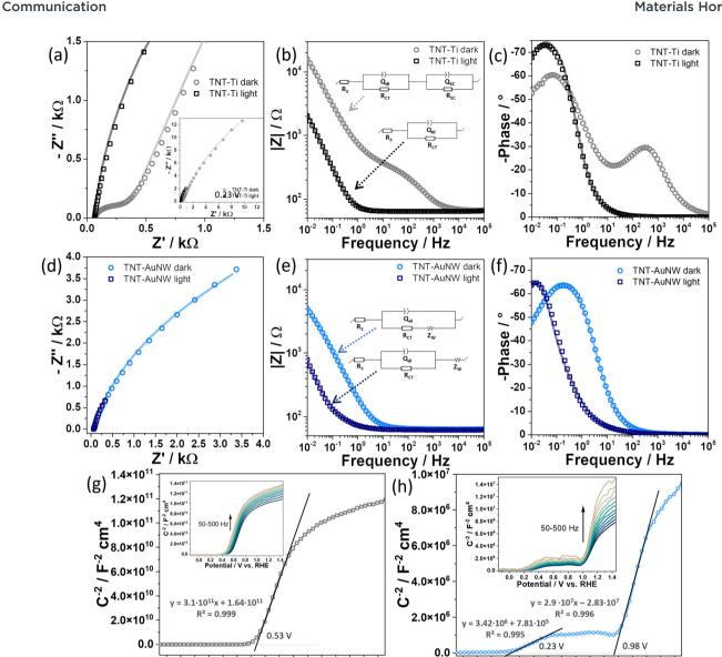
Fig. 6 (a and d) Nyquist and (b, c and e, f) Bode plots fitted with simulated equivalent circuits determined for TNT-Ti and TNT-AuNW, respectively. Empty symbols correspond to the experimental data; sold line correspond to the fitting obtained with equivalent circuits presented in (b and e). Mott-Schottky plots measured at a frequency range of 50-500 Hz for (g) TNT-Ti and (h) TNT-AuNW electrodes
