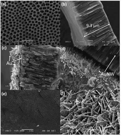
Fig. 2 SEM images of pristine anodic TiO<sub>2</sub> nanotube arrays after 20 minutes of 2<sup>nd</sup> step anodizing from (a) top view and (b) cross-section; and TNT-AuNW (c) cross-sectional view, (d) interface of AuNWs slightly detached from TNTs due to sample cutting, (e) top of the TNT-AuNW electrode (bottoms of TNTs), (f) flake-like morphology of its Au thin film (back side of the photoanode).
